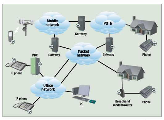
Figure 1- IP network endpoints
