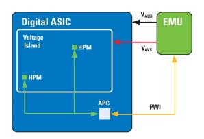
Figure 2. AVS Block Diagram
