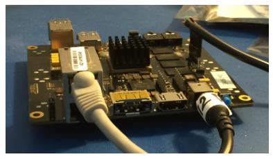
Figure 8. Connecting the Ethernet Cable
