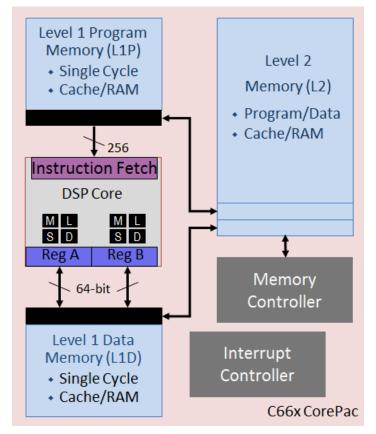
Figure 4. C66x Block Diagram
