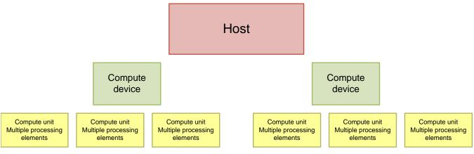
Figure 3. OpenCL Platform Model
