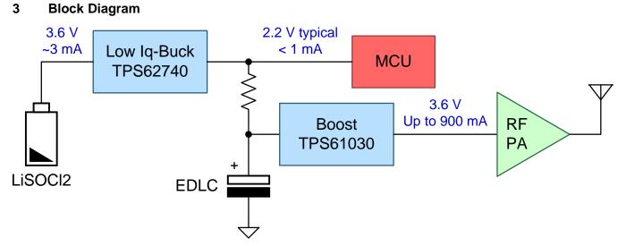
Figure 6. High Current Power Solution for Battery-Operated Meters Block Diagram
