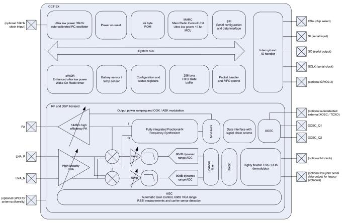
Figure 4. CC1120 Functional Block Diagram
