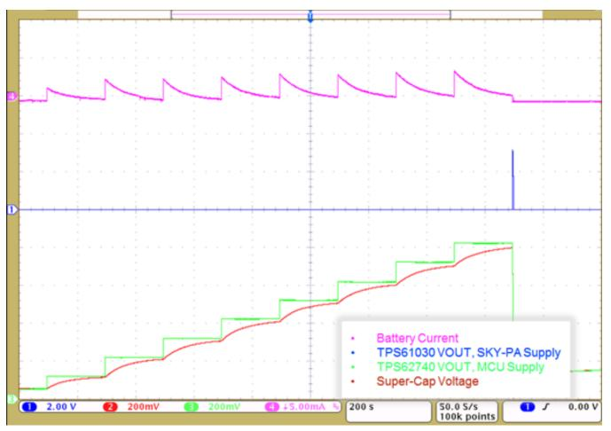
Figure 10. Transmission Sequence Including Energy Buffering
