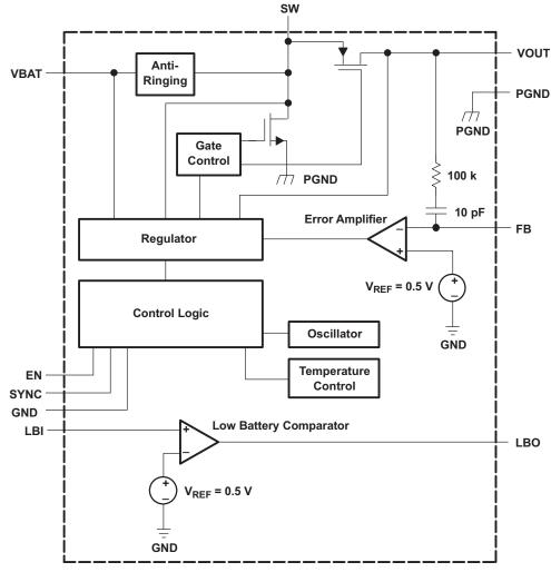
Figure 2. TPS61030 Block Diagram
