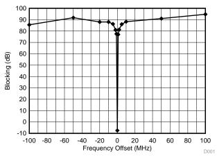
Figure 13. Nabef Blocking (Measured at Na Channel)
