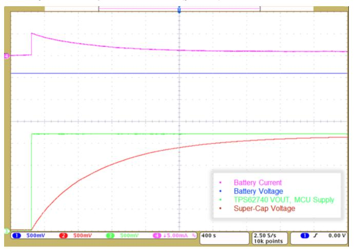
Figure 12. Startup Waveform for Initialization
