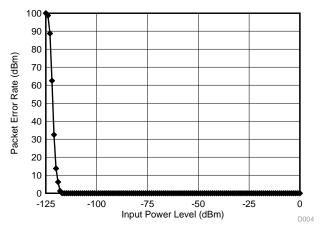
Figure 16. Ncd PER Plot (Measured at Nc Channel)
