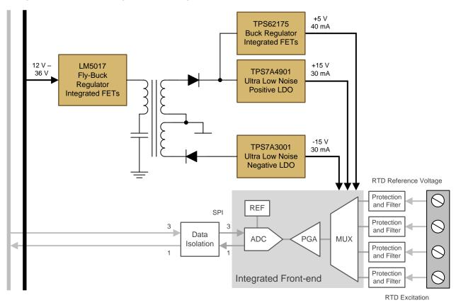
Figure 1. Generic Illustration of Analog Input Module
