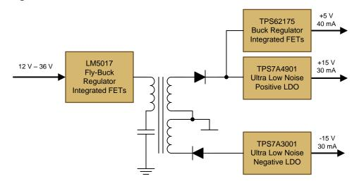
Figure 2. TIDA-00237 Isolated Power Supply Diagram for Analog Input Module
