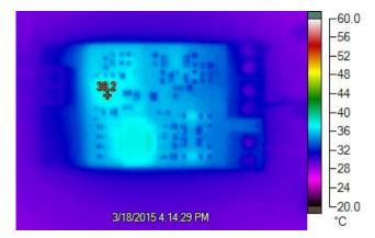
Figure 14. TIDA-00237 Thermal Analysis Full Load, V<sub>IN</sub> = 12 V
