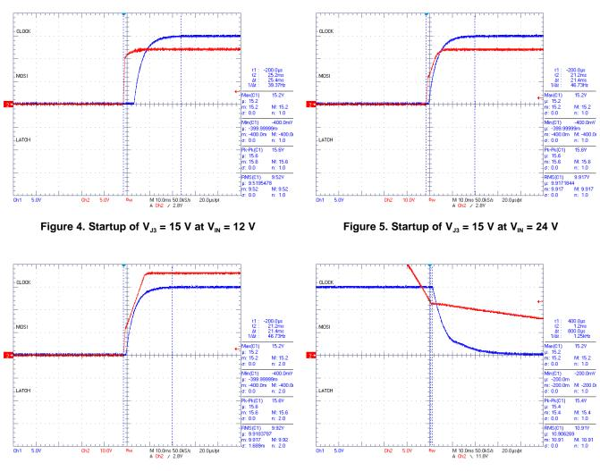
Figure 6. Startup of  $V_{J3}$  = 15 V at  $V_{IN}$  = 36 V
