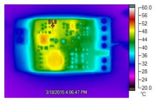
Figure 15. TIDA-00237 Thermal Analysis Full Load, V<sub>IN</sub> = 36 V
