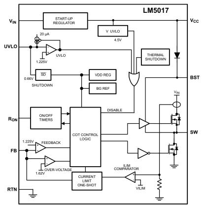
Figure 3. LM5017 Circuit Diagram
