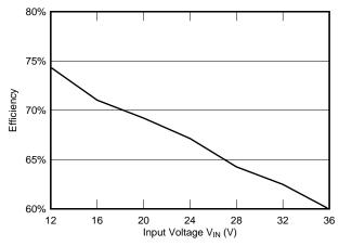
Figure 12. Overall Efficiency versus Input Voltage
