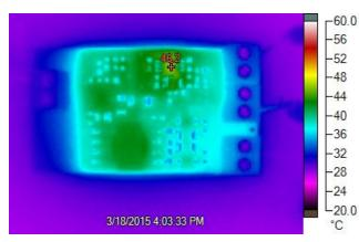
Figure 13. TIDA-00237 Thermal Analysis Full Load V<sub>IN</sub> = 24 V
