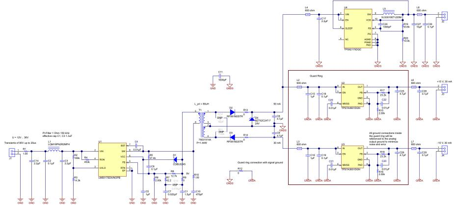
Figure 16. TIDA-00237 Schematic
