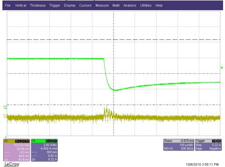
The waveform below shows the output voltage(in yellow, 10mV/div) after a 50% load-step of the output current(in green, 2A/div) from 5A to 10A. The timescale is 100us/div and the input voltage is 12.6V.
