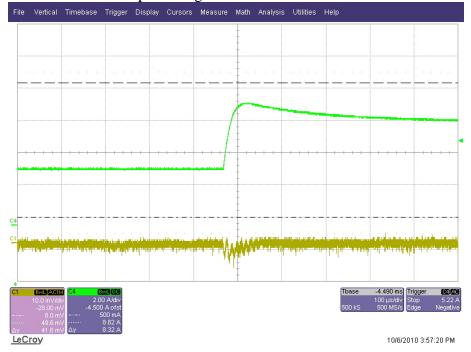
The waveform below shows the output voltage(in yellow, 10mV/div) after a 50% load-step of the output current(in green, 2A/div) from 10A to 5A. The timescale is 100us/div and the input voltage is 9V.
