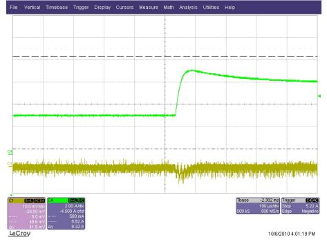
The waveform below shows the output voltage(in yellow, 10mV/div) after a 50% load-step of the output current(in green, 2A/div) from 10A to 5A. The timescale is 50us/div and the input voltage is 12.6V.
