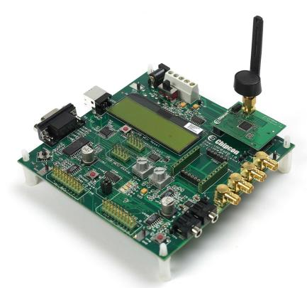
Figure 1 SmartRF04EB with CC2430EM
