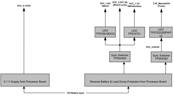
Figure 5. Power Supply Block Diagram
