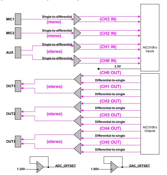
Figure 8 shows the block diagram of the analog audio circuits.
