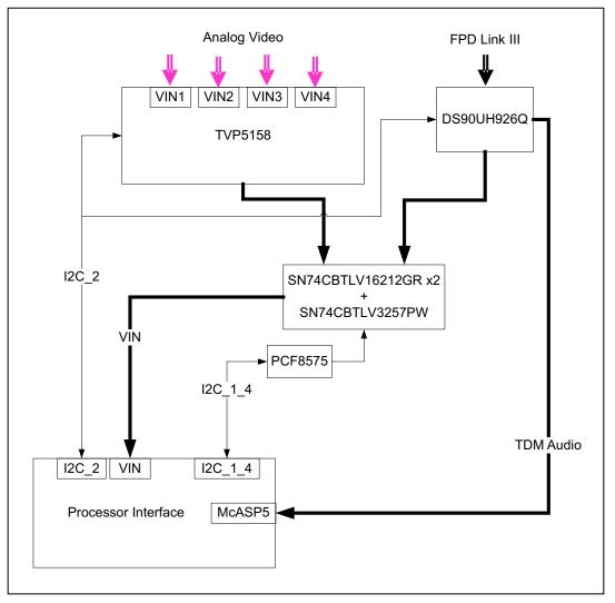
Figure 9. Video Processing Block Diagram
