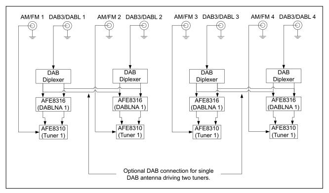
Figure 6. Radio Functional Block Diagram
