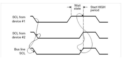
Figure 2-3 Synchronization of Two I<sup>2</sup>C Clock Generators During Arbitration
