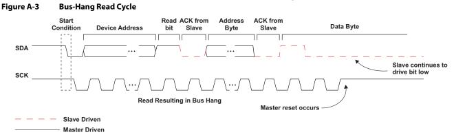
The master initiates a read in the normal fashion but a reset occurs while the SCK is high and the slave is driving the SDA low. The slave device will continue to drive SDA low waiting for the master to provide the next clock however the master has been reset and is no longer attempting to complete the read cycle. In addition, if the master attempts to access the bus after its reset has been released it will fail to arbitrate for control.
