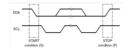
After a START condition and before a subsequent STOP condition, the I<sup>2</sup>C-bus is considered busy, and the bus busy (BB) bit of ICSTR is 1. Between a STOP condition and the next START condition, the bus is considered free, and BB is 0.
