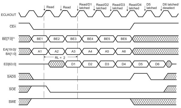
Figure 17. SBSRAM Six-Element Read Timing Diagram
