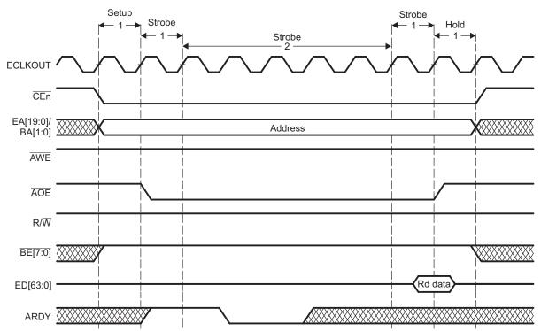
Figure 15. Asynchronous Read in WE Strobe Mode
