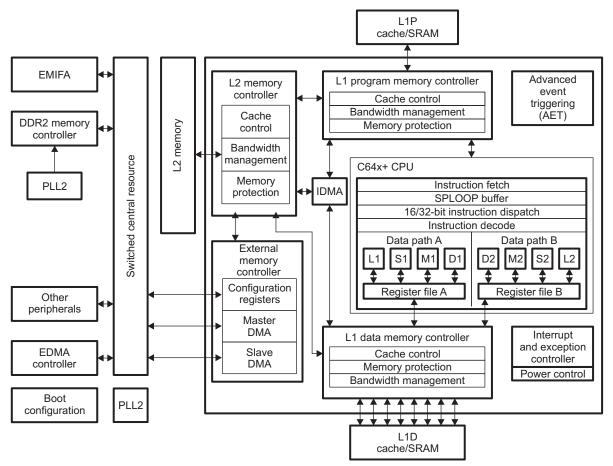
Figure 1. TMS320C645x DSP Block Diagram
