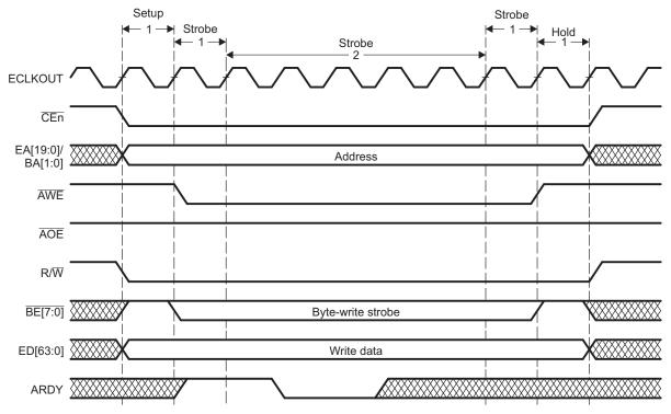
Figure 14. Asynchronous Write in WE Strobe Mode
