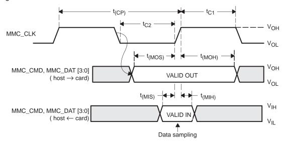
Figure 4. MMC/SD/SDIO ac Characteristics
