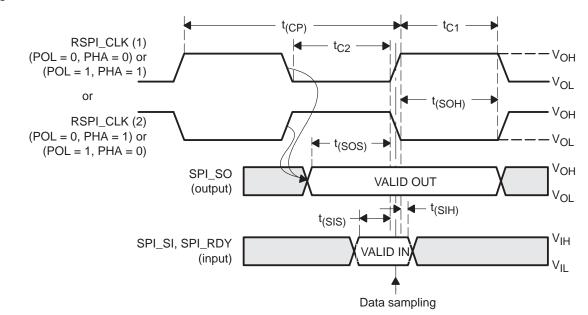
Figure 5. SPI ac Characteristics
