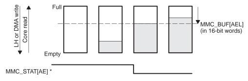
\* Non–DMA mode only. In DMA mode, the DMA RX request is asserted to its active level under identical conditions.
