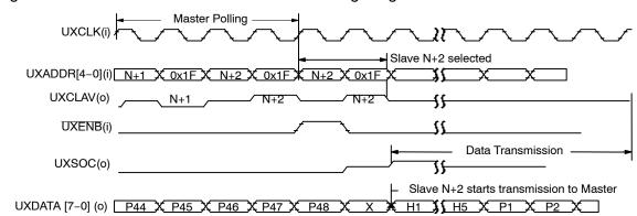
Figure 5. ATM Controller Slave Transmit Timing Diagram
