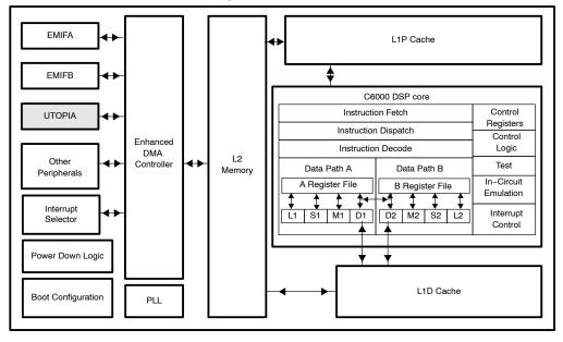
Figure 1. TMS320C64x DSP Block Diagram
