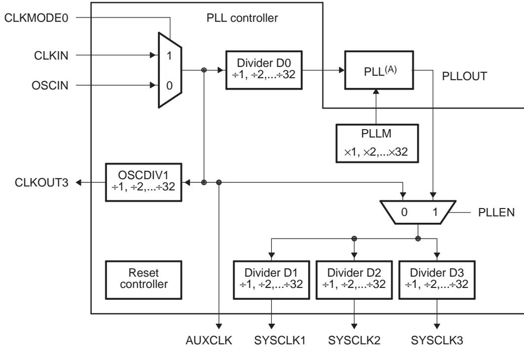
A See the device-specific data manual for more detail about the PLL.
