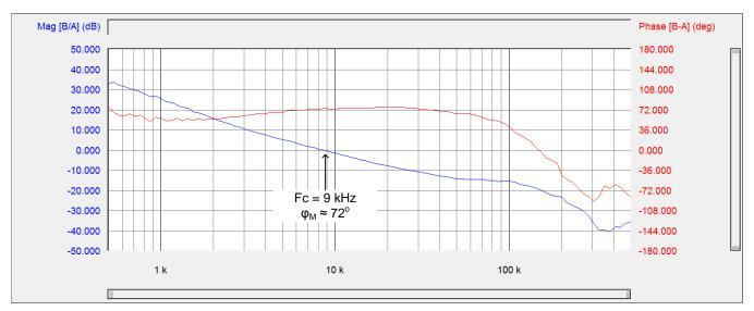
Figure 11. Bode Plot for  $V_{IN} = 12V$ ,  $I_{OUT} = 3A$
