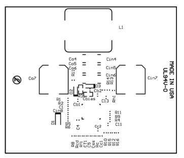
Figure 41. Bottom Layer Silkscreen (Bottom View)
