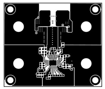
Figure 39. Bottom Copper (Bottom View)
