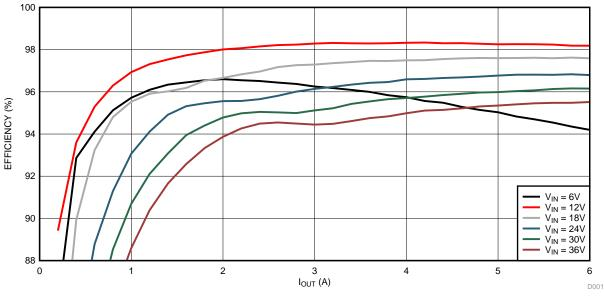
Figure 4. Efficiency vs. Output Current
