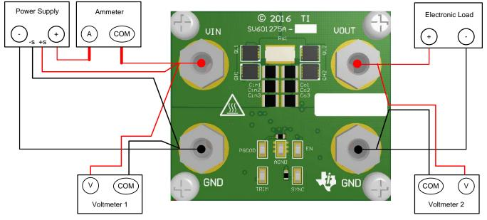
Figure 3. Test Setup Connection Diagram
