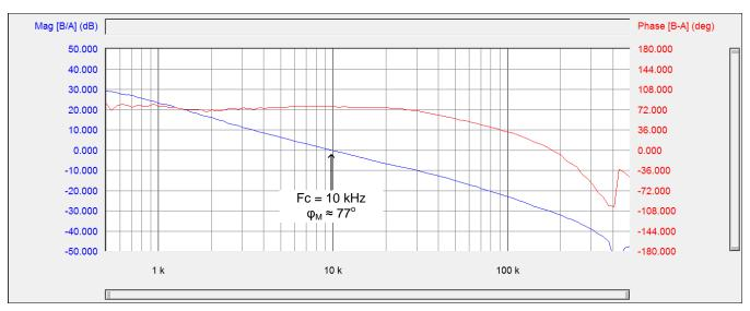
Figure 12. Bode Plot for  $V_{IN} = 24V$ ,  $I_{OUT} = 3A$
