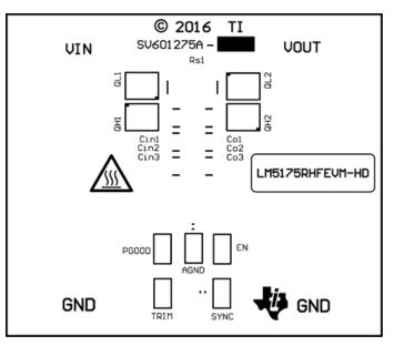
Figure 40. Top Layer Silkscreen (Top View)
