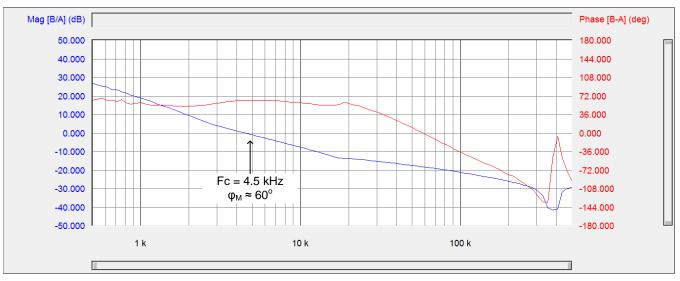
Figure 10. Bode Plot for  $V_{IN} = 6V$ ,  $I_{OUT} = 3A$
