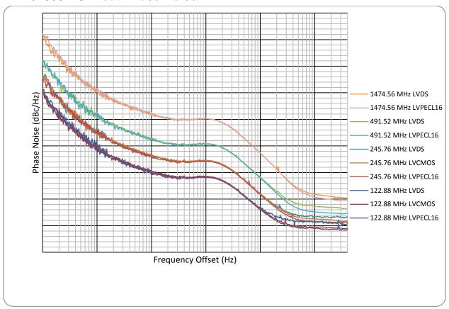
Figure 16: LMK04808B CLKout Phase Noise
