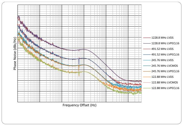
Figure 18: LMK04806B CLKout Phase Noise
