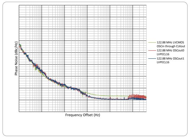
Figure 21: LMK04803B OSCout Phase Noise
