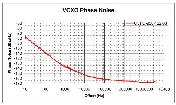
Figure 15: Crystek CVHD-950-122.88 MHz VCXO Phase Noise at 122.88 MHz
