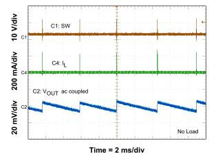
Figure 13. Output Voltage Ripple Eco-mode
