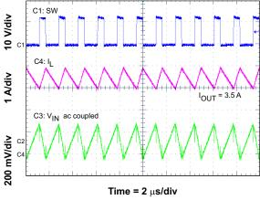
Figure 14. Input Voltage Ripple CCM
