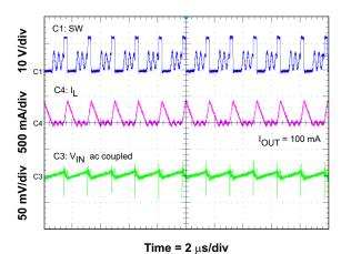
Figure 15. Input Voltage Ripple DCM
