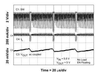
Figure 21. Low Dropout Operation
