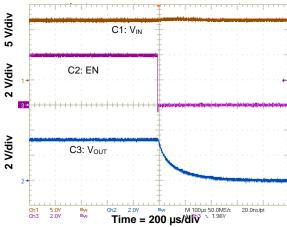
Figure 19. Shutdown Relative to VIN
