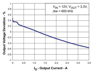
Figure 6. Regulation Versus Output Current
