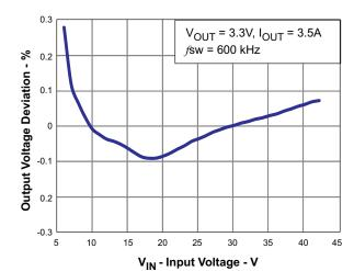
Figure 7. Regulation Versus Input Voltage
