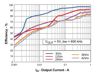
Figure 4. Efficiency Versus Load Current
