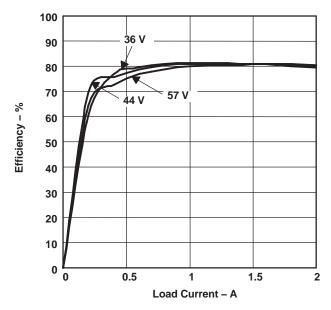
Figure 3. Typical 5-V PD End-to-End Efficiency
