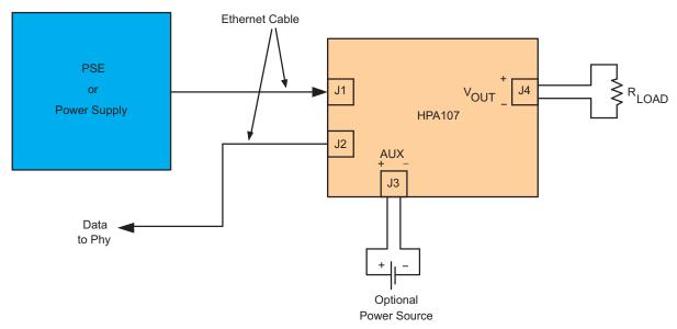
Figure 5. Typical Setup
