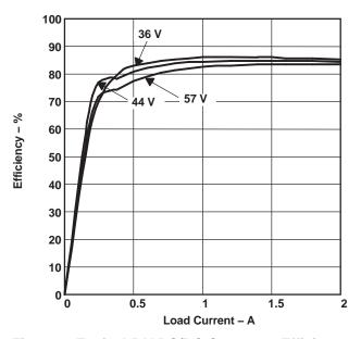
Figure 4. Typical 5-V DC/DC Converter Efficiency
