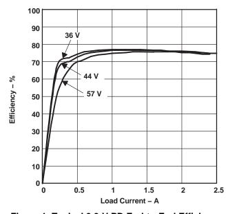
Figure 1. Typical 3.3-V PD End-to-End Efficiency
