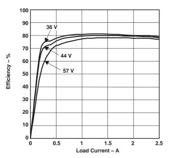
Figure 2. Typical 3.3-V DC/DC Converter Efficiency
