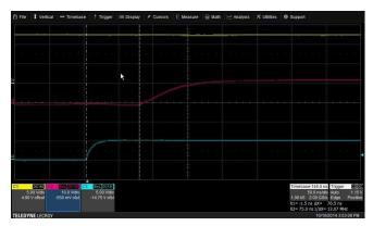
Figure 20. LI, LO Turn-On Propagation Delay
