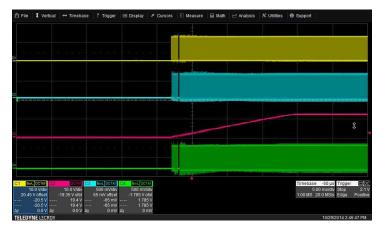
Figure 28. UCC28950 Burst-Mode Function During Soft Start
