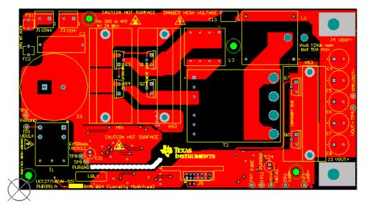
Figure 29. UCC27714EVM-551 Power Stage Top Layer Assembly Drawing (top view)
