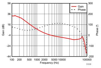
Figure 6. Loop Gain/Phase at 50 A,  $f_c = 2 \text{ kHz}$ , PM = 90 Degrees
