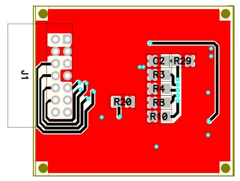
Figure 32. UCC27714EVM-551 Daughter Controller Card Bottom Layer Assembly Drawing (bottom view)
