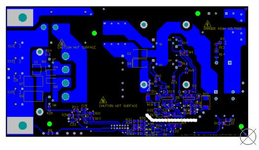
Figure 30. UCC27714EVM-551 Power Stage Bottom Layer Assembly Drawing (bottom view)
