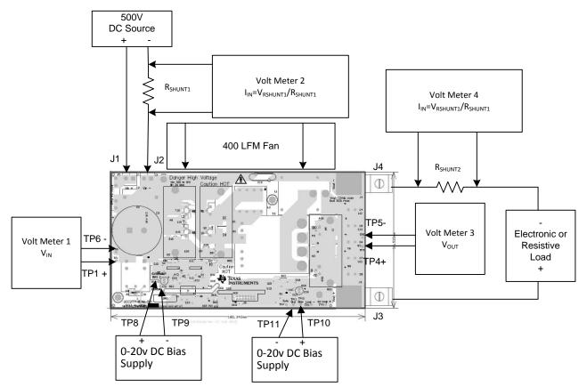
Figure 3. Test Setup to Measure Efficiency
