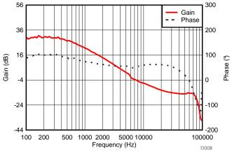
Figure 7. Loop Gain/Phase at 5 A,  $f_c = 6$  kHz, PM = 45 Degrees
