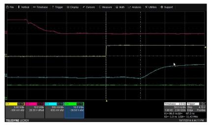
Figure 23. HI, HO Turn-On Propagation Delay
