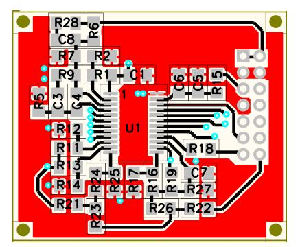
Figure 31. UCC27714EVM-551 Daughter Controller Card Top Layer Assembly Drawing (top view)
