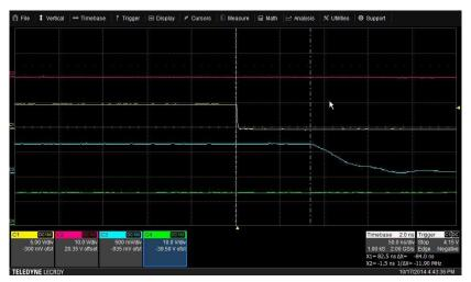
Figure 24. HI, HO Turn-Off Propagation Delay
