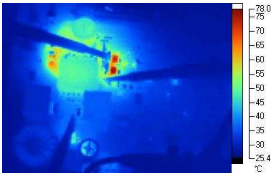
TOP Side Left side Power stage P_{out}=150\text{W} @ V_{out}=25\text{V}
