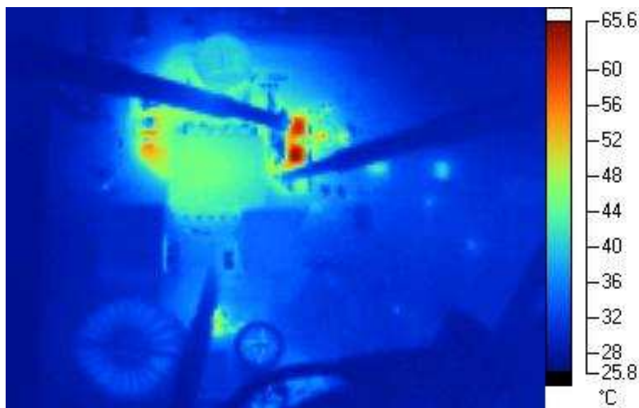
TOP Side Left side Power stage P_{out}=115\text{W} @ V_{out}=25\text{V} ( V_{IPWM}=60\% )
