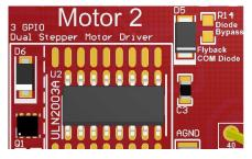
Figure 19. COM Diode Section With R14 Depopulated
