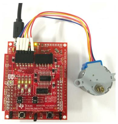
Figure 13. USB Powering a Single Motor (See NOTE)
