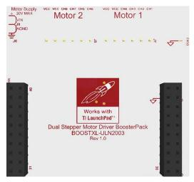
Figure 3. Bottom View of BOOSTXL-ULN2003
