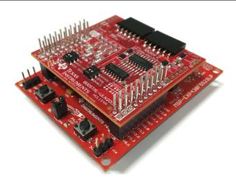
Figure 20. BoosterPack Connected to MSP430F5529 LaunchPad
