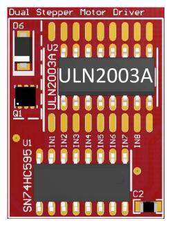
Figure 14. BoosterPack With ULN2003A
