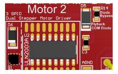
Figure 18. Board Image of COM Diode Section
