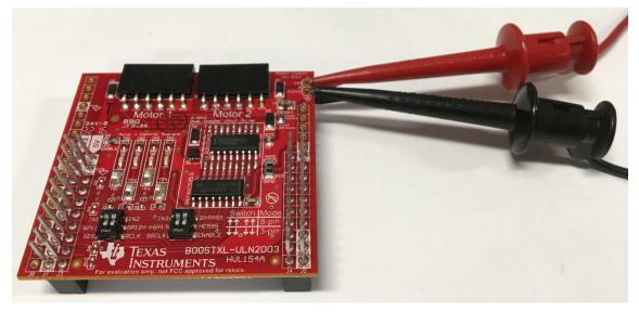
Figure 11. External Supply Connected to Motor Supply Pins
