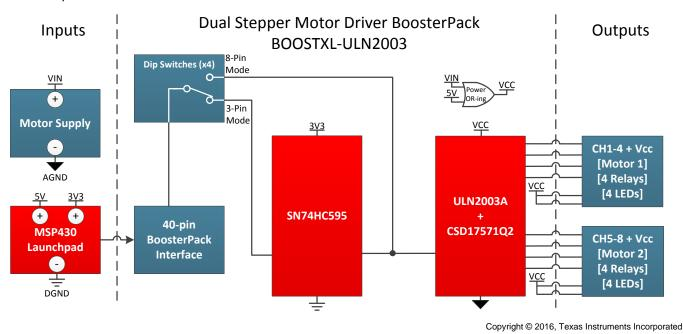
Figure 5. BOOSTXL-ULN2003 Block Diagram
