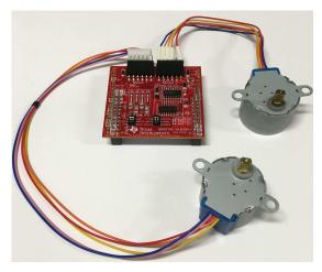
Figure 21. BoosterPack With Two Stepper Motors
