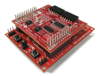
Figure 1. BOOSTXL-ULN2003 Connected to MSP-EXP430F5529LP
