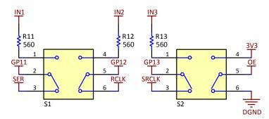
Figure 8. Schematic View of Switches
