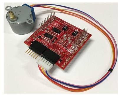
Figure 22. BoosterPack with Motor and Male Expansion Header
