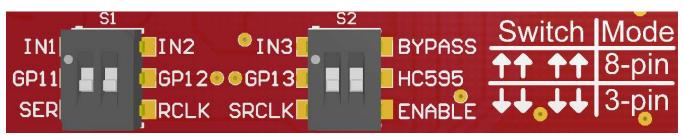
Figure 7. Board Image of Switches
