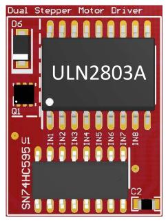
Figure 15. BoosterPack With ULN2803A
