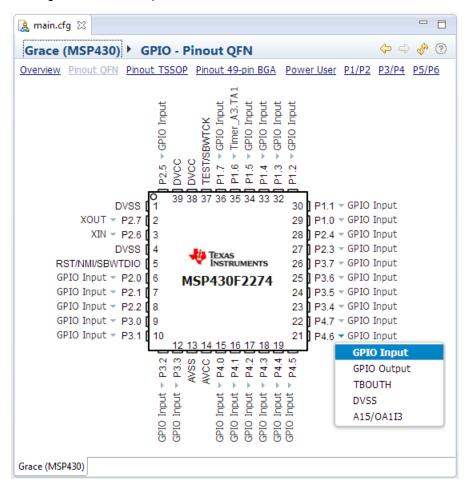
Figure 10. G2xx/F2xx GPIO Configuration, Pinout View
