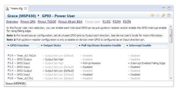
Figure 11. G2xx/F2xx GPIO Configuration, Power User View
