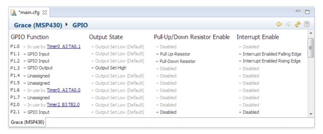
Figure 14. FR5xx GPIO Configuration, Power User View
