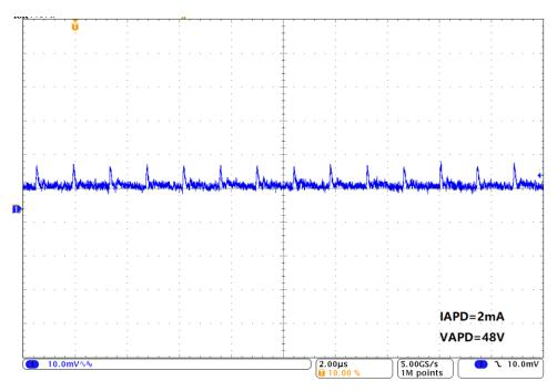
Figure 4. APD Bias Voltage Ripple at 2-mA APD Current ( $V_o = 48 V$ )
