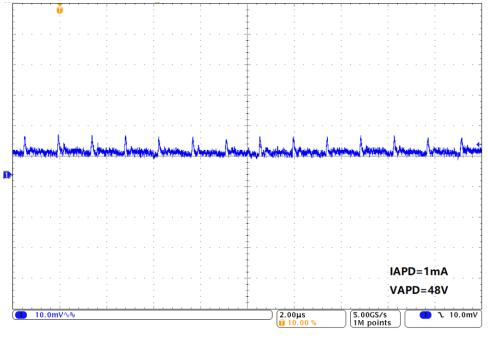
Figure 3. APD Bias Voltage Ripple at 1-mA APD Current ( $V_o = 48 V$ )
