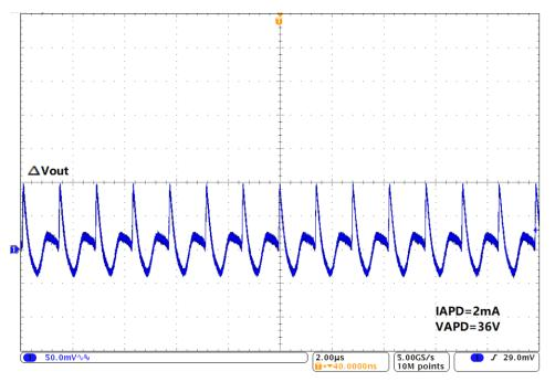
Figure 6. Output Voltage Ripple at 2-mA APD Current ( $V_o = 36 V$ )
