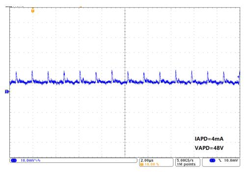
Figure 5. APD Bias Voltage Ripple at 4-mA APD Current ( $V_o = 48 V$ )
