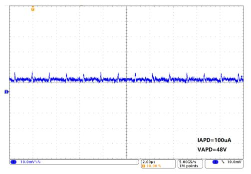
Figure 2. APD Bias Voltage Ripple at 100- $\mu$ A APD Current (V<sub>o</sub> = 48 V)
