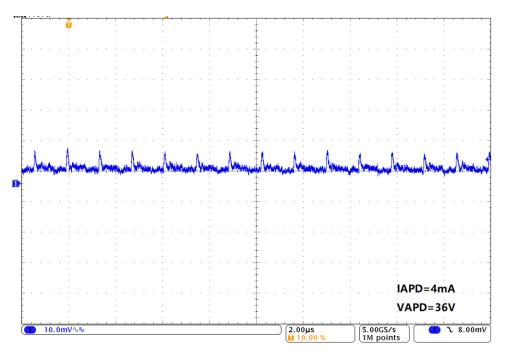
Figure 8. APD Bias Voltage Ripple at 4-mA APD Current ( $V_o = 36 V$ )
