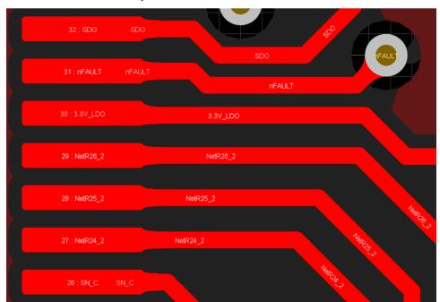
图 26. Teardrops Used on Transitions From Vias to Pads
