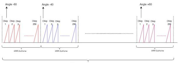
图 10. Beamsteering Scheme in BSD, LCA, and TJA Reference Design
