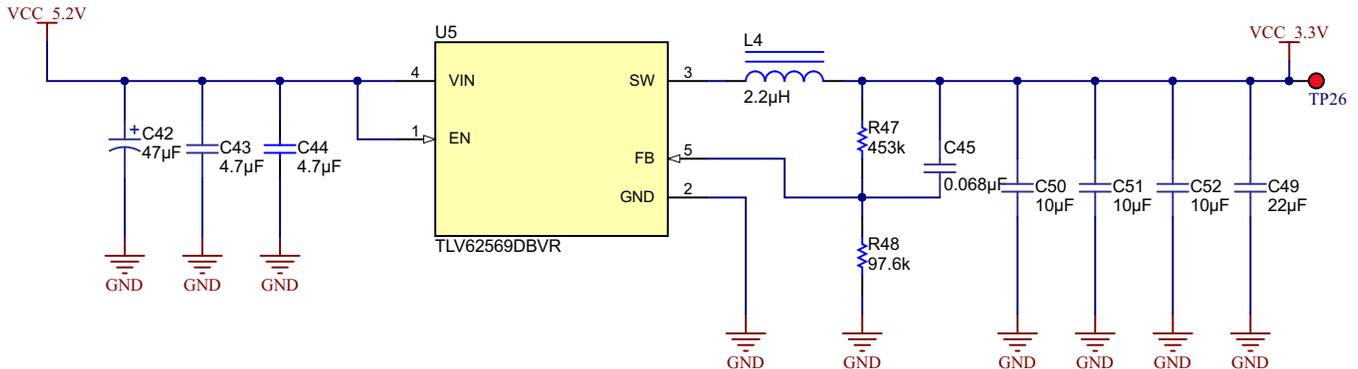
图 16 shows the switching circuit generating 3.3 V using the TLV62569 from the 5.2-V DC/DC Converter. 3.3 V is provided to the following:
