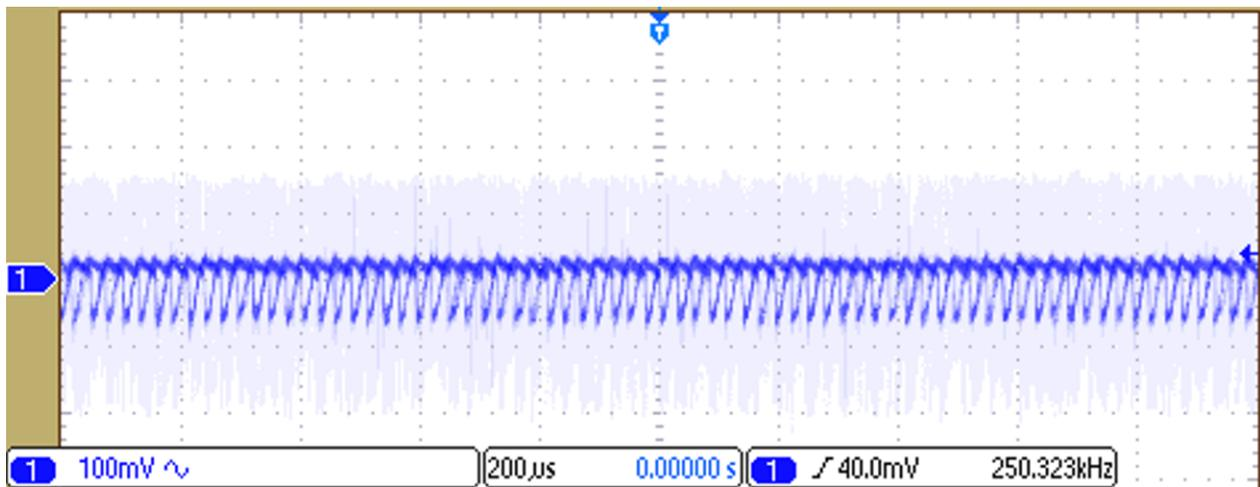
图 31. Output Ripple Voltage of 5 V Supply for Input Voltage of 3.7 V, and Input Current of 120 mA
