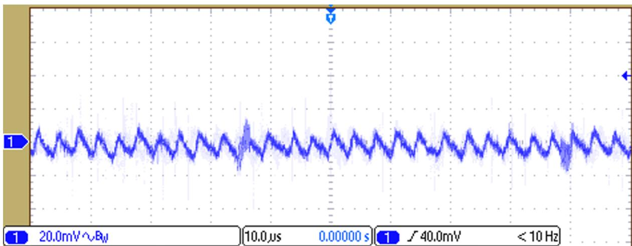
图 32. Output Ripple Voltage of 3.3 V Supply for Input Voltage of 3.7 V, and Input Current of 120 mA
