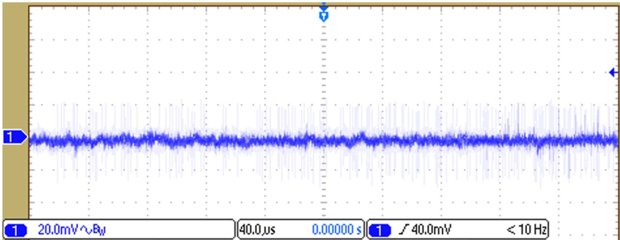
图 33. Output Ripple Voltage of 3.3 V Supply for Input Voltage of 3.7 V, and Input Current of 120 mA
