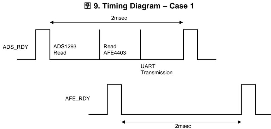
图 10 shows ADS1292R and AFE4403 Read and UART transmission (AFE4403 RDY comes while reading ADS1292).
