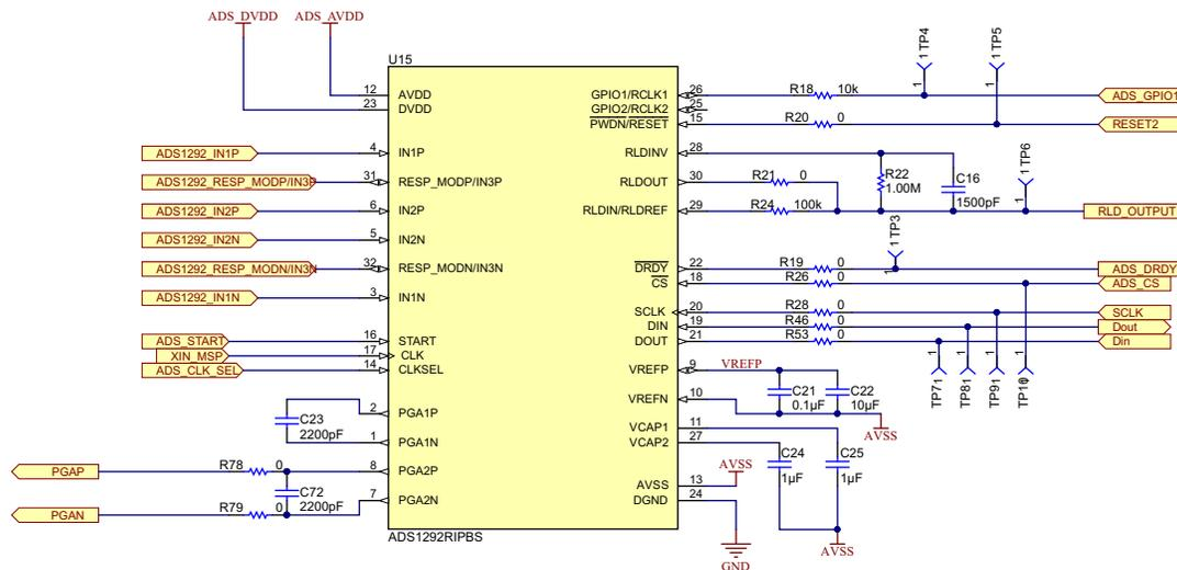
图 5. ECG Subcircuit – Decoupling Capacitor and Ferrite Bead
