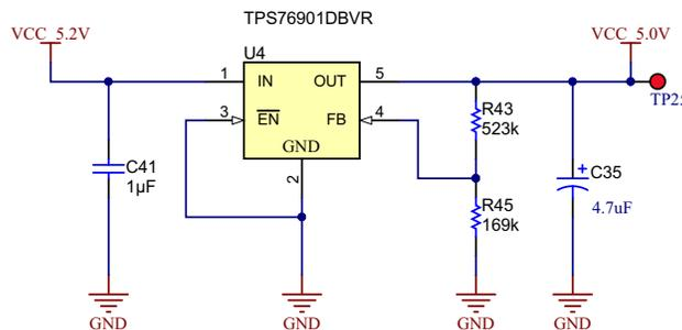
图 14 shows the LDO circuit generating 5 V from a 5.2-V input using the TPS76901. The 5 V provides the LED\_DRV\_SUP and TX\_CTRL\_SUP of the AFE4403 IC. The TPS76901 device is an ultra-low power 100-mA low-dropout linear regulator.
