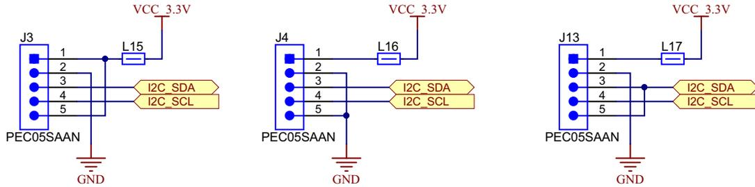
图 19 shows the connection to the temperature sensor TMP117. Three TMP117 temperature sensors are used for accurate measurement. Interface is from the I2C to the MCU. ADD0 pin is the fifth pin and connects to GND, V1, and SDA lines to select the unique slave address.
