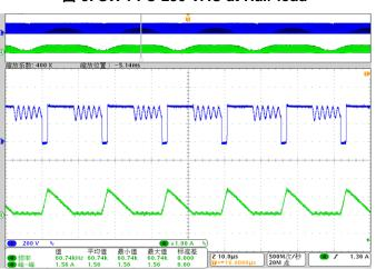
图 9. SW-PFC-230 VAC at Half-load
