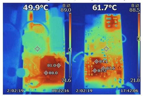
图 23. Thermal Image at 115-V AC, 60-Hz Input, 20-V, 5-A Output
