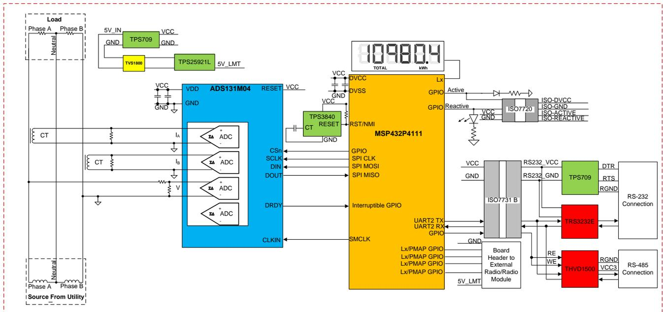
In the diagrams, a current sensor connects to the current channels and a simple voltage divider is used for the corresponding voltage. The CT has an associated burden resistor that must be connected at all times to protect the measuring device. The selection of the CT and the burden resistor is made based on the manufacturer and current range required for energy measurements.
