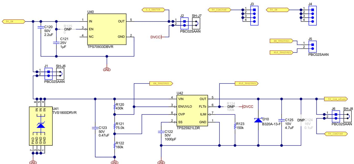
The current-limiting functionality in this design is performed by the TPS25921L e-Fuse device, which powers the load connected to the J3 header from the source connected to the header on J4. For proper operation, use 5 V as the voltage provided by the source connected to J4. There is a TPS70933 LDO that can be used to generate the 3.3-V rail for the ADS131M04 device and MSP432 MCU from the 5 V applied at J4 so that only one input rail is necessary.
