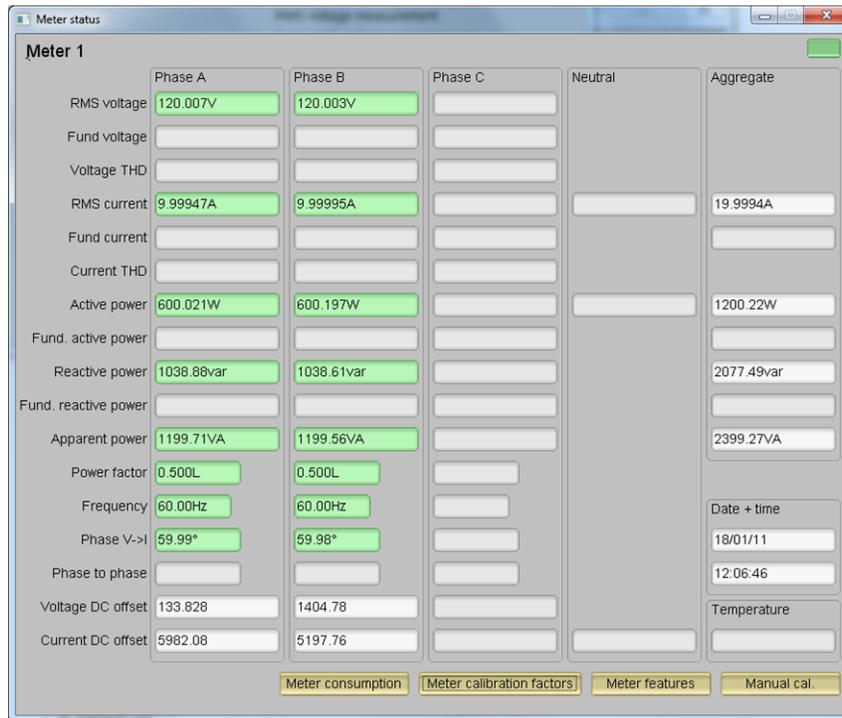
From the results window, the total-energy consumption readings can be viewed by clicking the *Meter Consumption* button. After the user clicks this button, the *Meter events and consumption* window pops up, as 图 29 shows.
