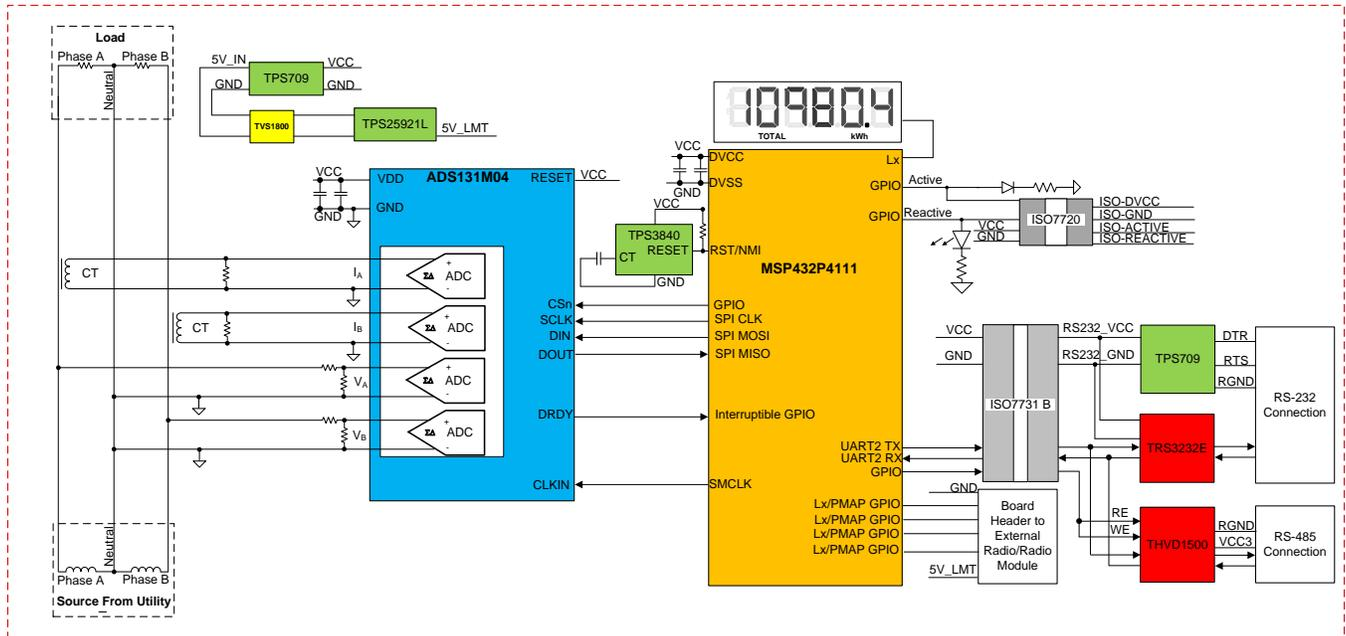
图 2. TIDA-010037 Block Diagram, One-Voltage Configuration
