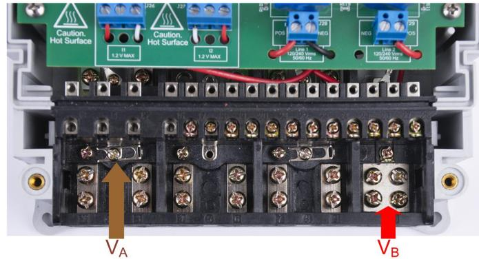
图 22 shows the connections from the front view.  $V_A$  and  $V_B$  correspond to line A and line B.  $I_{A+}$  and  $I_{A-}$  correspond to the current inputs for line A while  $I_{B+}$ , and  $I_{B-}$  correspond to the current inputs for line B.
