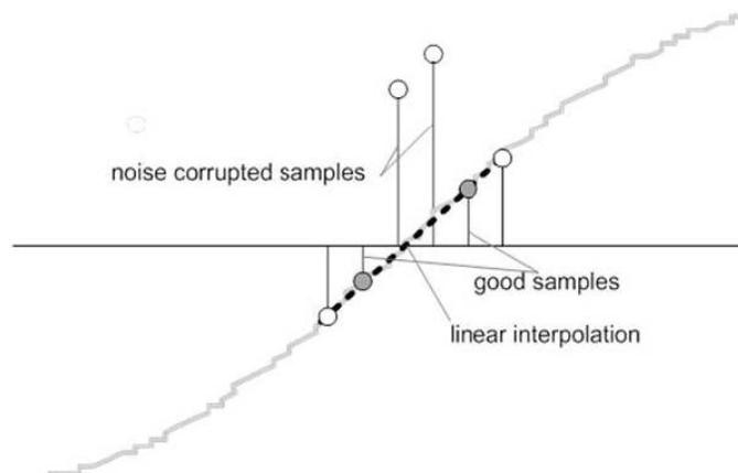
Because noise spikes can also cause errors, the application uses a rate-of-change check to filter out the possible erroneous signals and make sure that the two points are interpolated from genuine zero crossing points. For example, with two negative samples, a noise spike can make one of the samples positive, thereby making the negative and positive pair appear as if there is a zero crossing.
