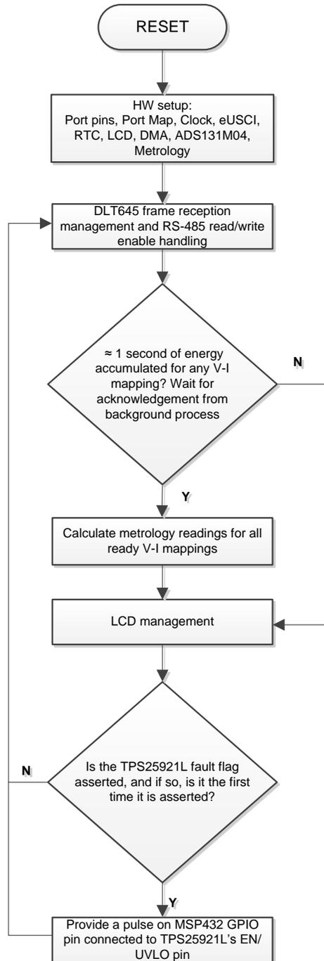
The initialization routines involve the setup of the MSP432 general purpose input/output (GPIO) port pins and associated port map controller; MSP432 clock system; MSP432 USCI\_A0 for UART functionality; MSP432 RTC module for clock functionality; MSP432 LCD; MSP432 DMA; ADS131M04 registers; and MSP432 metrology variables.
