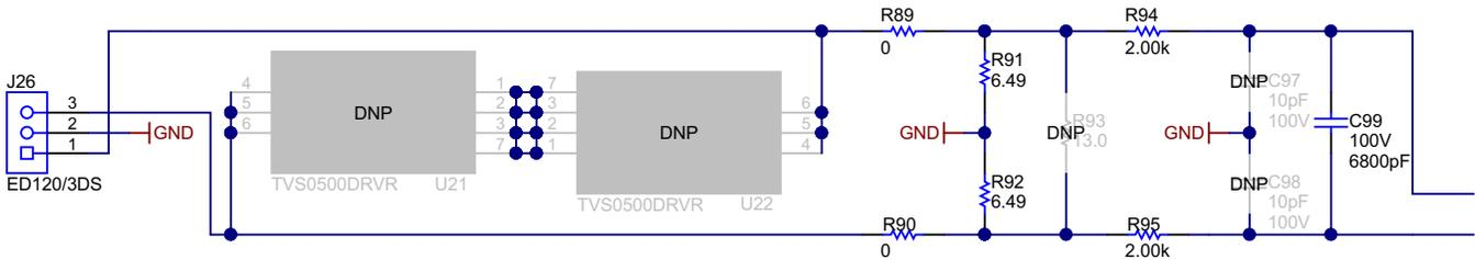
The analog front end for current consists of footprints for electromagnetic interference filter beads (R89 and R90), burden resistors for current transformers (R91 and R92), and an RC low-pass filter (R94, R95, C97, C98, and C99) that functions as an anti-alias filter. There are also footprints (U21 and U22) that can be replaced with the TVS0500 for supplemental protection from surges, if required.
