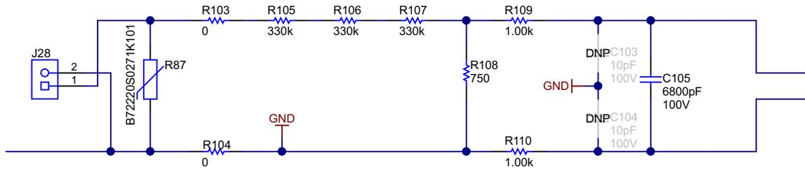
In the analog front end for voltage, there consists a spike protection varistor (R87), footprints for electromagnetic interference filter beads (resistor footprints R103 and R104), a voltage divider network (R105, R106, R107, and R108), and an RC low-pass filter (R109, R110, C103, C104, and C105).
