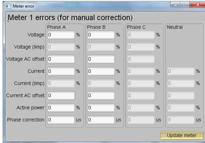
4. Calculate the correction values for each voltage and current. The correction values that must be entered for the voltage and current fields are calculated using 公式 17:
