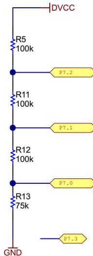
If the LCD is not needed and P7.0, P7.1, or P7.2 is to be used for some other functionality, such as communication to an external radio module, remove the resistors in 图 7 and use software to implement the desired custom functionality.
