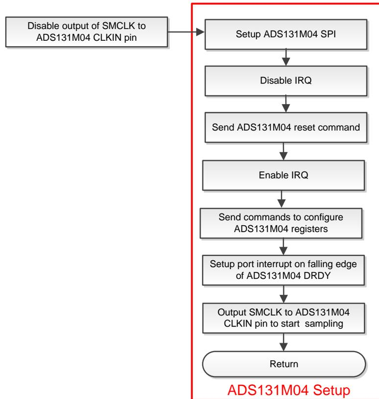
Before setting up the ADS131M04 device, the modulator clock of the ADS131M04 is disabled to prevent the ADS131M04 from generating new samples while trying to set it up. The modulator clock is disabled by disabling the SMCLK output of the MSP432 MCU, which is fed to the CLKIN pin of the ADS131M04. Disabling the SMCLK output only needs to be done after calibration and not after an MSP432 MCU reset event since the SMCLK clock output is automatically not output after the MSP432 MCU resets.
