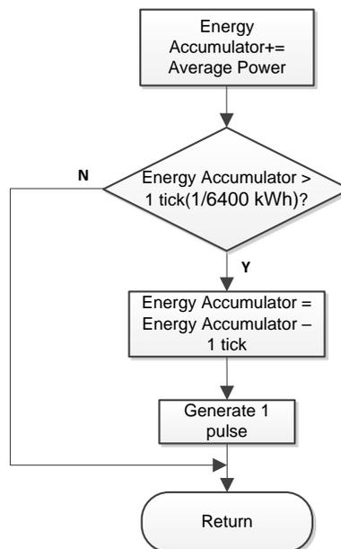
The average power is in units of 0.001 W and a 1-kWh threshold is defined as:
