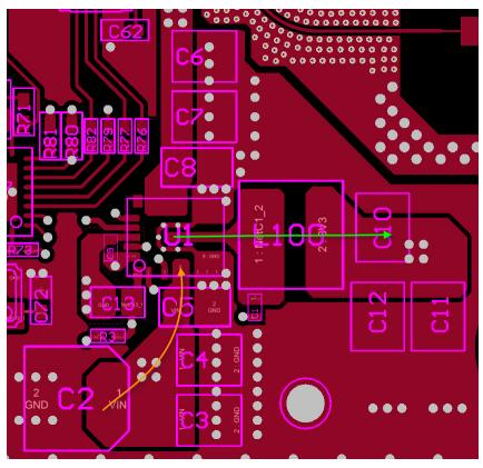
图 19. Current Paths Through Switching Converter
