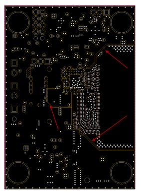
图 5. Cuts in Layer 2 Ground Plane
