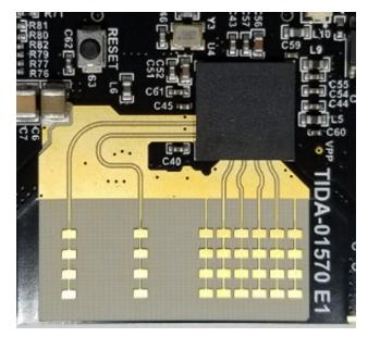
图 7. Antenna as Appears on PCB
