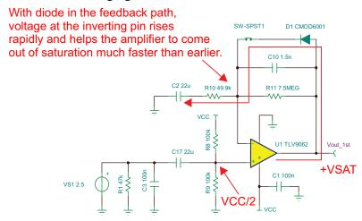
图 15. Power-on Settling Time Simulation With Diode
