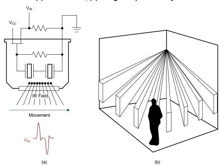
图 2. (a) Fresnel Lens, (b) Wedge-Shaped Sensory Patterns
