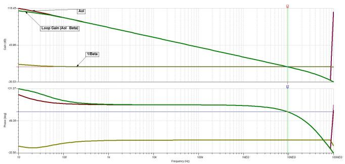
Stage-4 is exactly the same as stage-3, so the phase margin also remains the same. 图 16, 图 18, and 图 20 show the small signal stability frequency response of the circuit. As 图 17, 图 19, and 图 21 show, all amplifier stages (Stage-1, Stage-2, Stage-3, and Stage-4) of the signal conditioning circuit are stable with a phase margin of greater than 72°, respectively.
