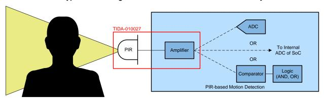
Any PIR-based motion detection circuit consists of several elements each with specific functions.
