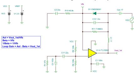
图 16. Test Circuit for Stage-1 Stability Analysis
