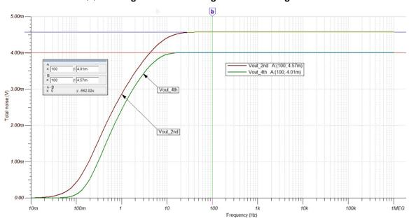
图 10. Integrated Noise of Signal Conditioning Circuit
