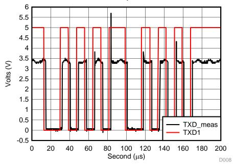
图 26. TXD Master Simulation Results Compared to Actual Cable Measurements
