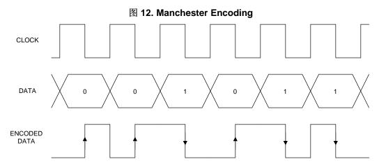
13 demonstrates a Manchester encoded signal for a sequence of constant 1's and 0's. In both cases, the encoded signal is always transitioning.
