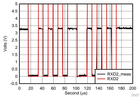
图 28. Bus Node At Input To Slave Simulation Results Compared to Actual Cable Measurements
