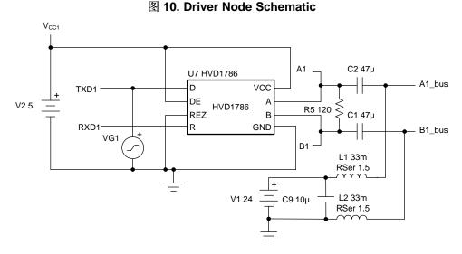
As  $\boxtimes$  11 shows, a coupling network consists of a capacitor that allows the AC signal through while blocking the DC voltage and an inductor which passes the DC voltage but blocks the AC signal. In transmission line environments the impedance of the capacitor ( $Z_c$ ) is chosen to be much less than the characteristic impedance of the cable,  $Z_0$ , and the impedance of the inductor ( $Z_L$ ) is chosen to be much greater than  $Z_0$ :
