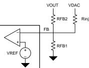
To create an adjustable DC voltage a PWM signal is run through a second order Sallen key low pass filter. The output DC voltage is adjusted by changing the input PWM duty cycle. See 3.2 <sup>††</sup> for a graph of PWM duty cycle to output voltage.
