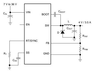
图 9. Application Circuit, 4-V Output
