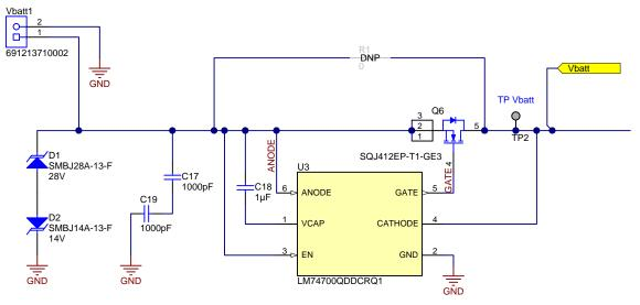
图 7. TIDA-020001 Schematic: Input Protection
