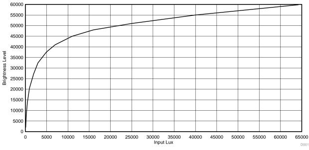
图 21 shows the ambient input lux to backlight brightness curve used for this design.
