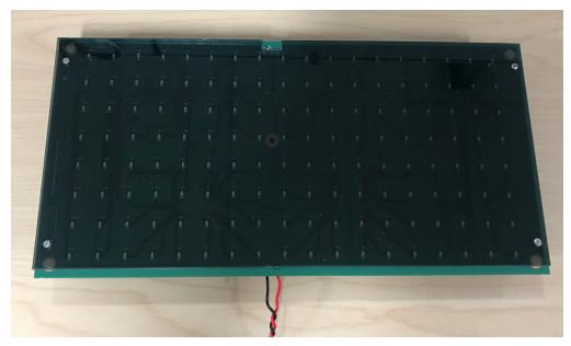
图 18. TIDA-020001 With Acrylic Light Attenuator
