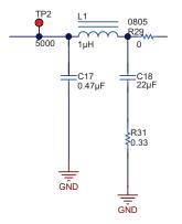
图 8. TIDA-020001 Schematic: PI Filter
