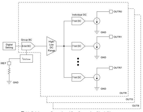
图 14. Brightness Control and Dot Correction Block Diagram
