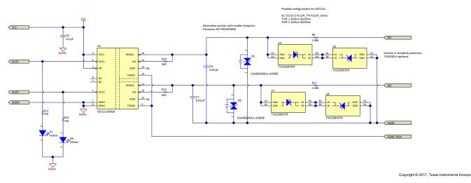
图 5. Schematic of Input Stage ISO1212
