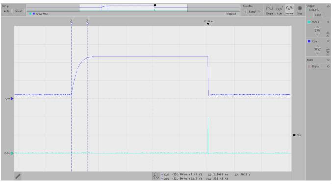
图 17. Single Broken Wire Detection,  $R_{pullup}$  = 100 k $\Omega$  - V\_cap (2), ChOut (1)
