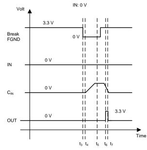
**\boxtimes** 9. Broken Wire Detection With Intact Wire and IN = 0 V
