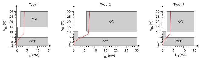
图 7. Switching Characteristics for IEC 61131-2 Type 1, 2, and 3 Proximity Switches
