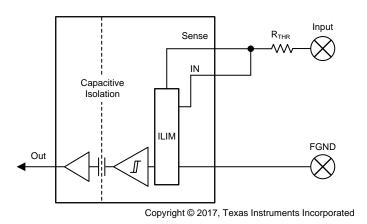
图 2. Functional Block Diagram of ISO121x
