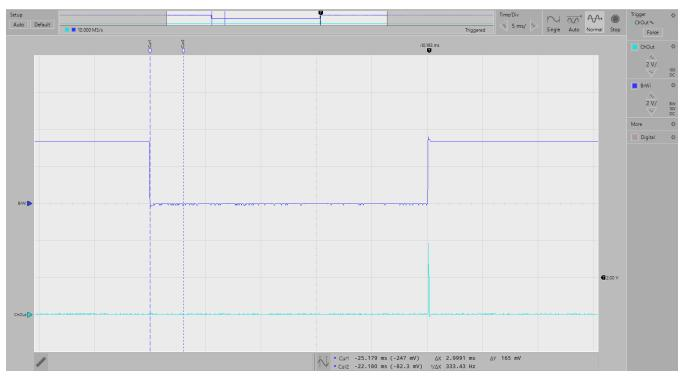
图 14. Group Broken Wire Detection,  $R_{pullup}$  = 800 kΩ/Channel - ChOut (2), BrWi (1)
