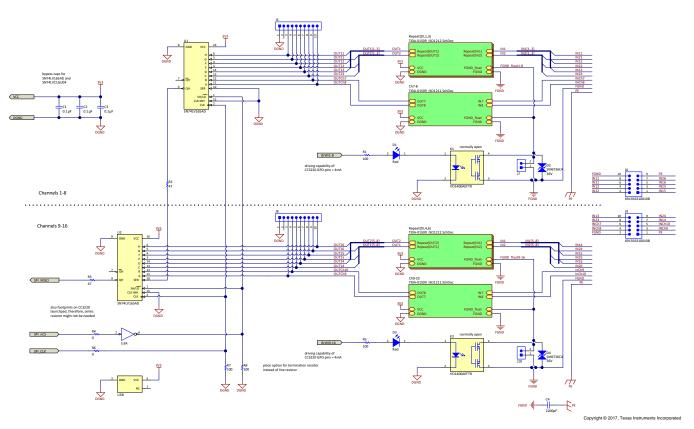
图 6. Schematic of Floating Ground to Field Ground (FGND) Connection With Optical Switch
