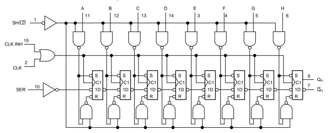
图 3. Functional Block Diagram of SN74LV165A
