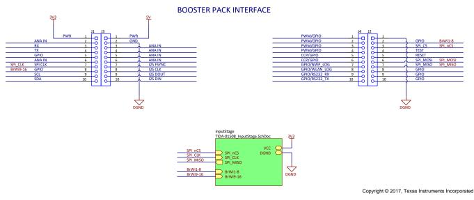
图 12. Schematic of LaunchPad Interface
