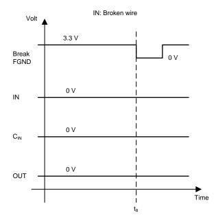
图 10. Broken Wire Detection With Broken Wire
