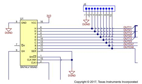
图 11. Schematic of Parallel and Serial Readout Options for Output Signals
