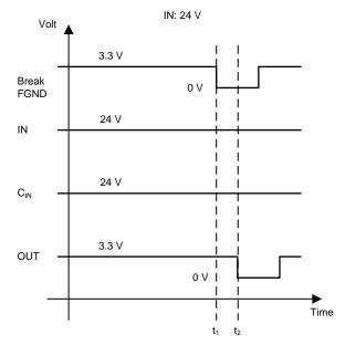
图 8. Broken Wire Detection With Intact Wire and IN = 24 V
