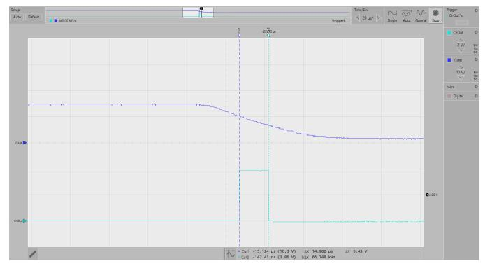
图 19. Single Broken Wire Detection, V = 14.9 V,  $R_{pullup}$  = 100 k $\Omega$  - V\_cap (2), ChOut (1)
