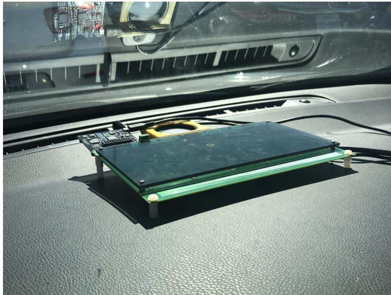
图 33. TIDA-01008 Outdoor Brightness—Front Dash of Vehicle
