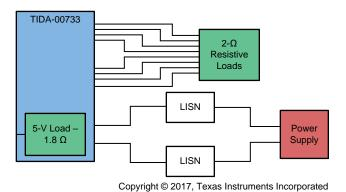
图 28. Test Setup Block Diagram for EMI Tests
