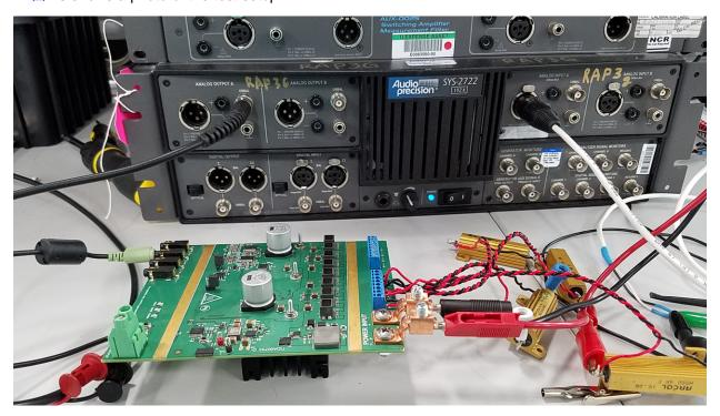
图 26. Test Setup for Power Output and Total Harmonic Distortion and Noise Tests
