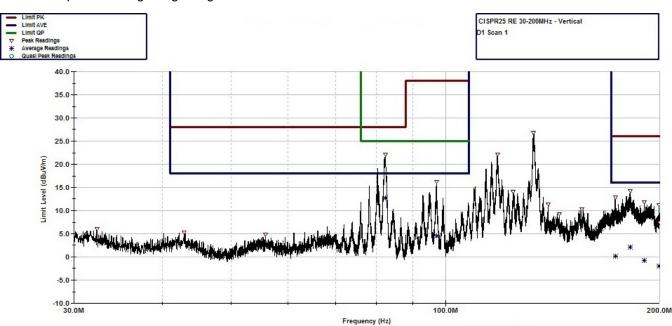
图 37. CISPR 25 Radiated Emissions: 30 MHz to 200 MHz, Vertical Antenna Orientation
