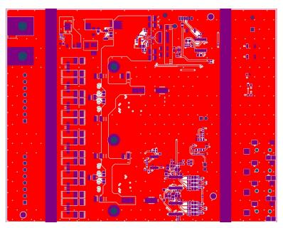
图 42. TIDA-00733 Top Circuit Board—Top Layer
