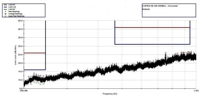
图 38. CISPR 25 Radiated Emissions: 200 MHz to 1 GHz, Horizontal Antenna Orientation, Ambient Scan
