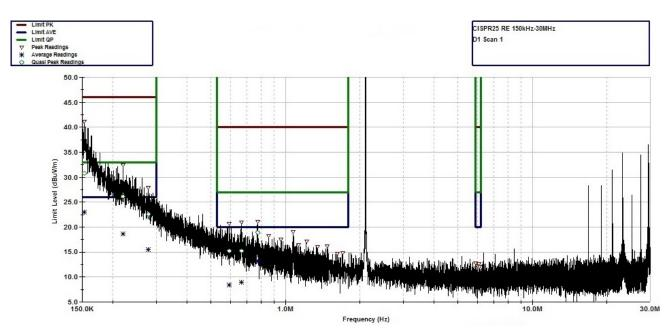
图 33. CISPR 25 Radiated Emissions: 150 kHz to 30 MHz
