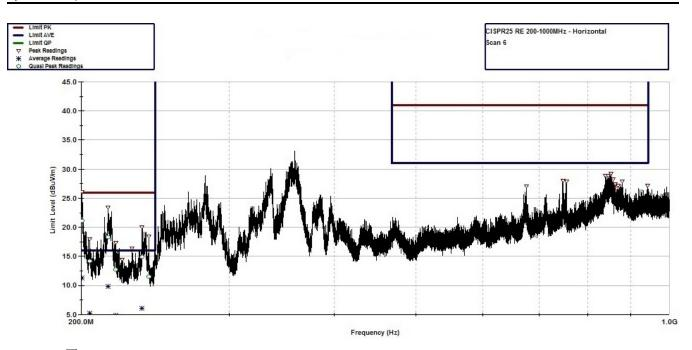
图 40. CISPR 25 Radiated Emissions: 200 MHz to 1 GHz, Horizontal Antenna Orientation
