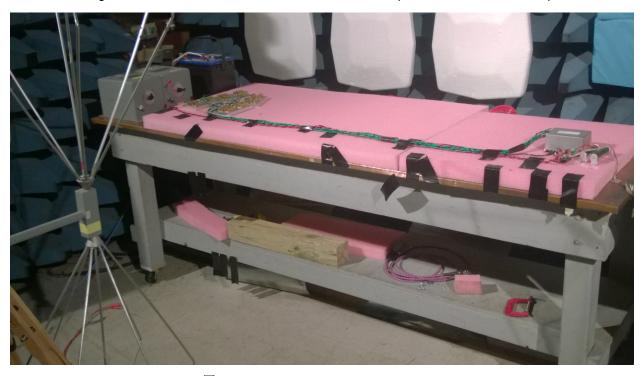
图 29. Radiated Emissions Test Setup
