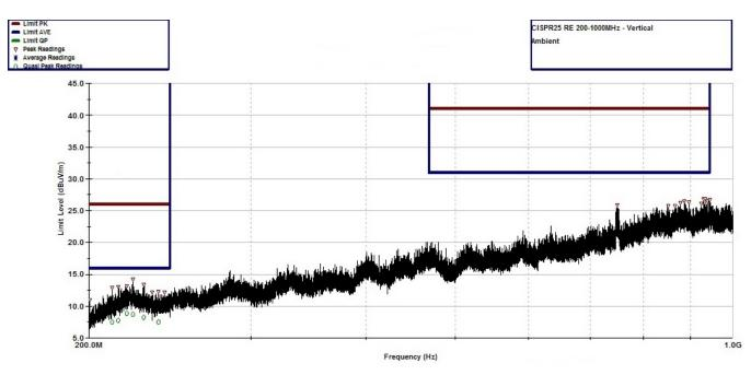
图 39. CISPR 25 Radiated Emissions: 200 MHz to 1 GHz, Vertical Antenna Orientation, Ambient Scan
