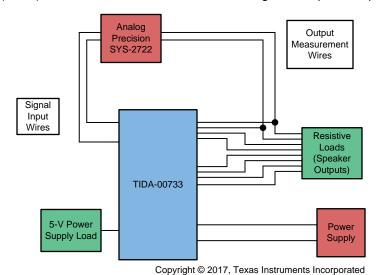
图 25. Test Setup Block Diagram for Power Output and THD Tests
