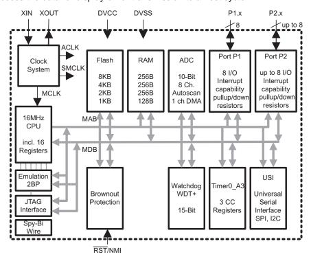
图 10. MSP430G2332 Functional Block Diagram
