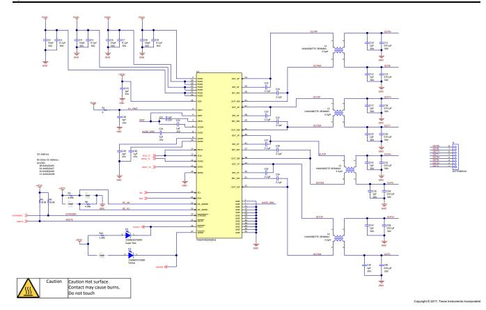
图 19. TAS6424-Q1 Class-D Power Audio Amplifier Circuits (Part 1 of 2)
