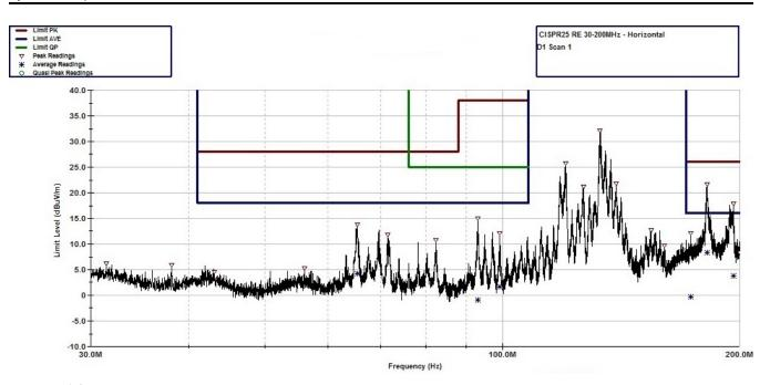
图 36. CISPR 25 Radiated Emissions: 30 MHz to 200 MHz, Horizontal Antenna Orientation
