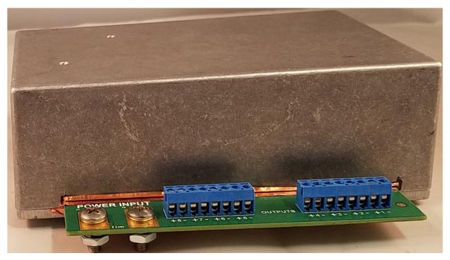
图 27. TIDA-00733 in Metal Box for EMI Tests
