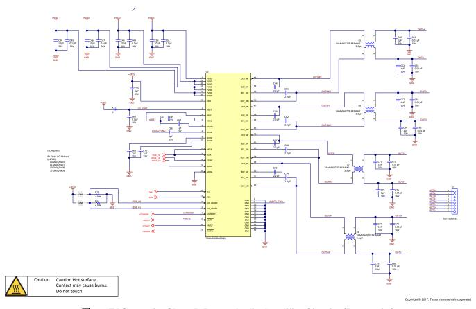
图 20. TAS6424-Q1 Class-D Power Audio Amplifier Circuits (Part 2 of 2)
