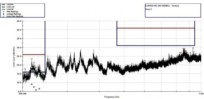
图 41. CISPR 25 Radiated Emissions: 200 MHz to 1 GHz, Vertical Antenna Orientation
