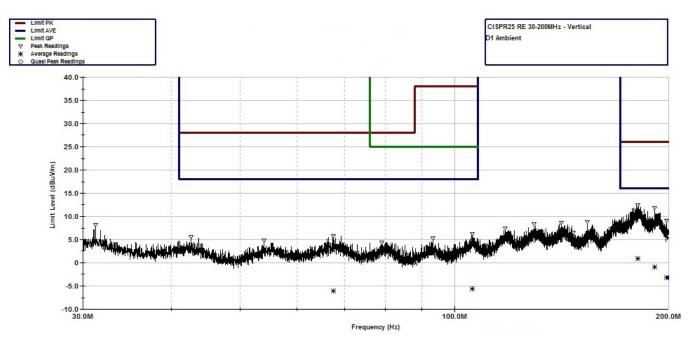
图 35. CISPR 25 Radiated Emissions: 30 MHz to 200 MHz, Vertical Antenna Orientation, Ambient Scan
