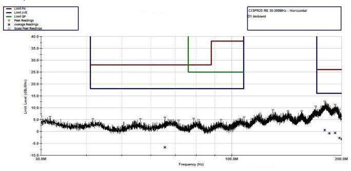
图 34. CISPR 25 Radiated Emissions: 30 MHz to 200 MHz, Horizontal Antenna Orientation, Ambient Scan
