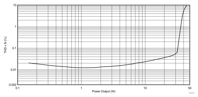
图 30. Power Output (W) vs THD + Noise (%) into 2  $\Omega$
