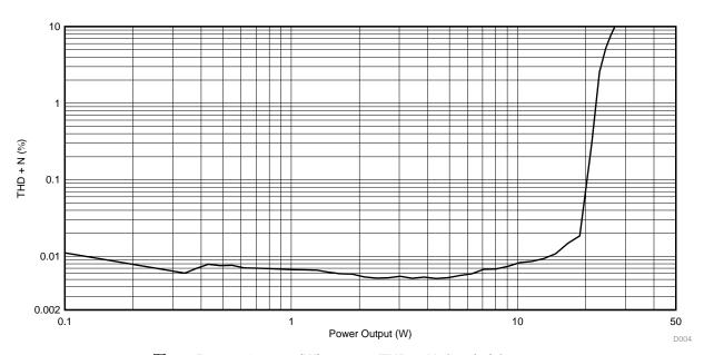
图 31. Power Output (W) versus THD + Noise (%) into 4  $\Omega$
