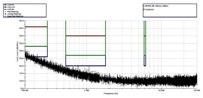
图 32. CISPR 25 Radiated Emissions: 150 kHz to 30 MHz, Ambient
