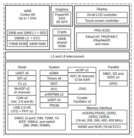
图 6. AM3359 Functional Block Diagram
