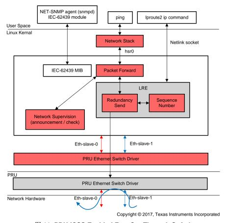
图 11. PRU-ICSS Enabled Fast Cut-Through Switch
