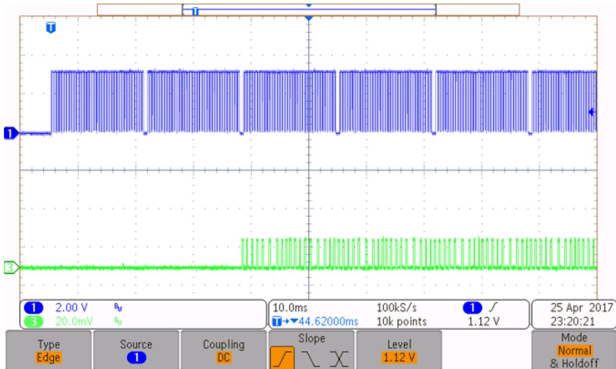
图 18. Two Frames of Delay at 60 Hz
