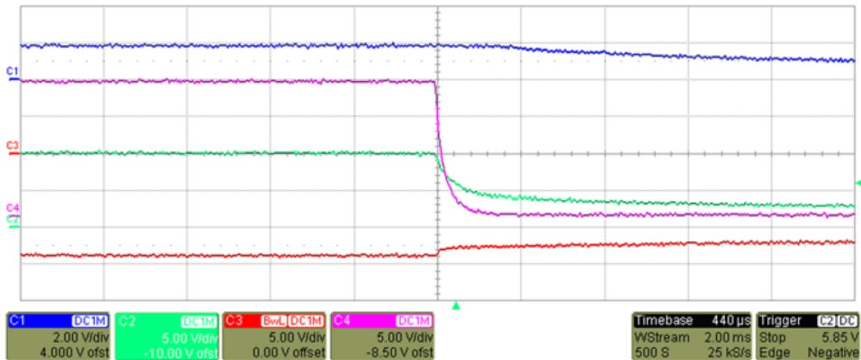
图 16. DMD Shutdown Power Sequencing
