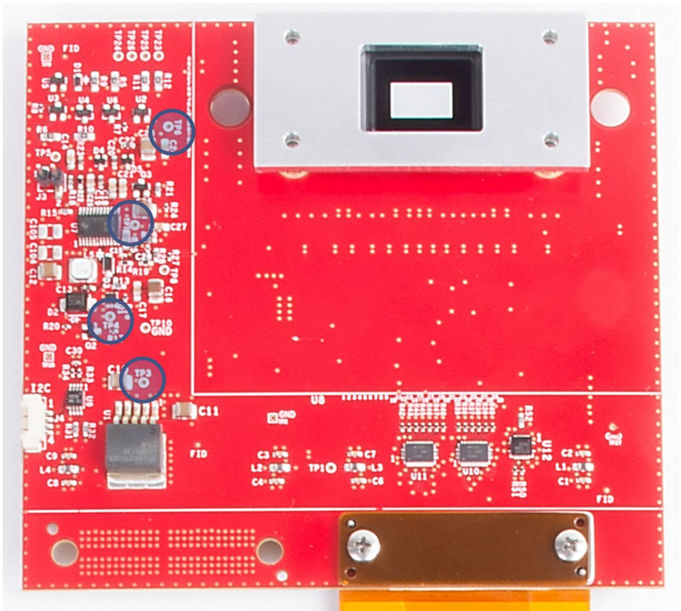
图 13. DMD Board Voltage Test Points
