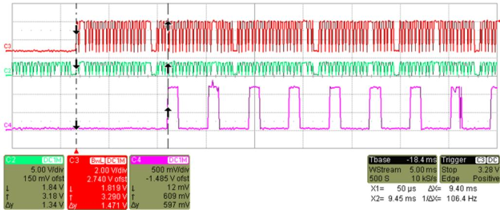
图 21. One Frame of Delay at 120 Hz
