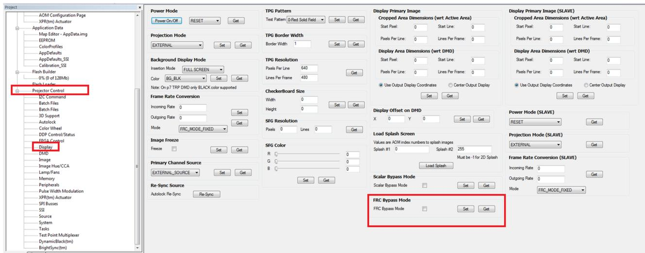
图 12. Enabling Low Latency Mode in DLP Composer™ Lite GUI
