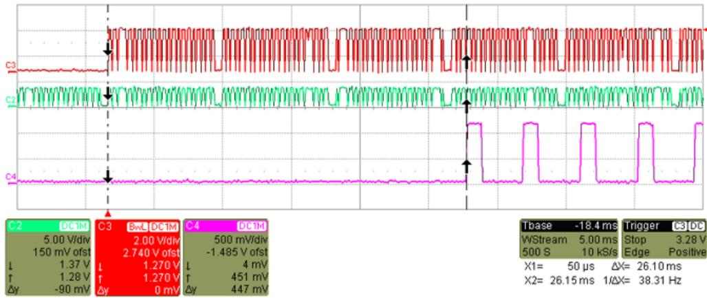
图 19. Three Frames of Delay at 120 Hz
