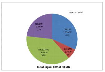
图 31. TIDA-01013 AFE (THS4551) and ADC Power Consumption
