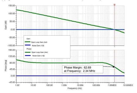
图 8. OPA191 TINA-TI Stability Simulation Results
