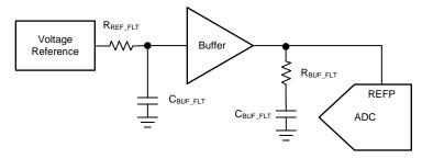
图 14. Simplified Schematic of Reference Driver
