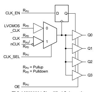
图 5. LMK00804 Simplified Schematic
