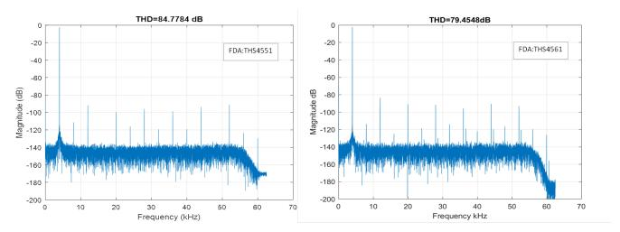
图 30. TIDA-01013 Fast-Fourier Transform for 10-V<sub>P</sub>, 4-kHz Sine Wave Input
