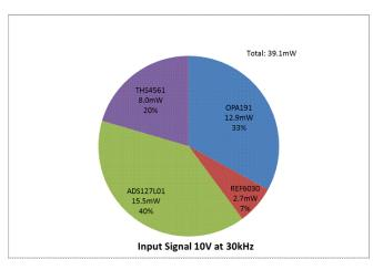
图 32. TIDA-01013 AFE (THS4561) and ADC Power Consumption
