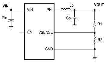
图 3. TPS560200 Simplified Schematic
