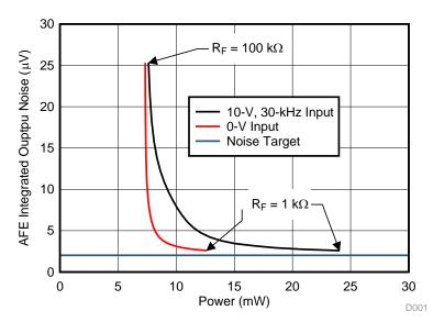
图 22. TIDA-01013 AFE Integrated Output Noise versus Power Plot
