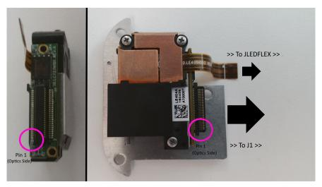
图 3. Overview of Connection for 0.2 nHD Optical Engine
