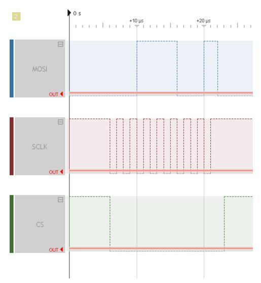
图 12. Example SPI Waveform for SN74HC595 Programming
