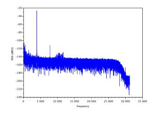
图 28. PSD for -37-dBFS Input at 3.9 kHz
