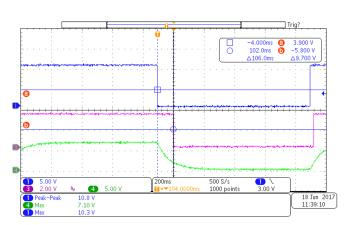
图 31. Short-Circuit Detection Delay
