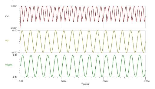
图 17. ICC Current Consumption for Whole Chain
