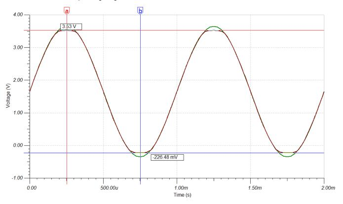
图 10. Overvoltage Clipping by Input Protection Diodes
