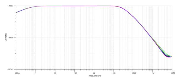
图 13. AC Transfer Characteristics of Signal Chain
