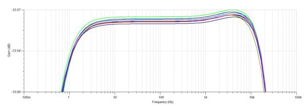
图 14. Signal Chain Passband at -12-dB Gain Setting
