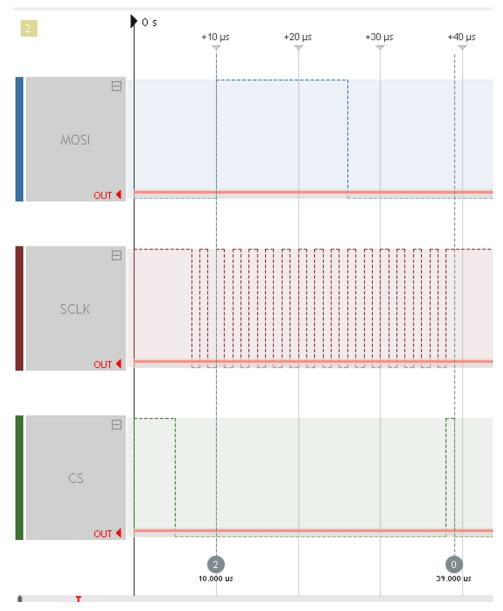
图 11. Example SPI Waveform for DAC5311 Programming
