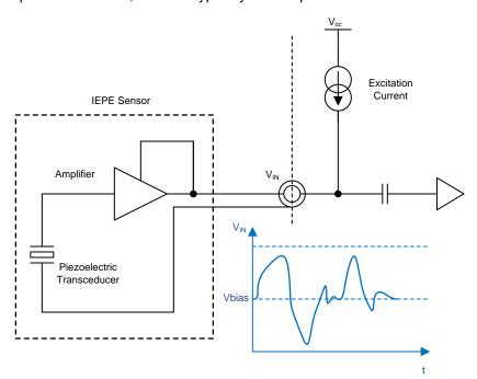
图 7. IEPE Sensor Conceptual Circuit
