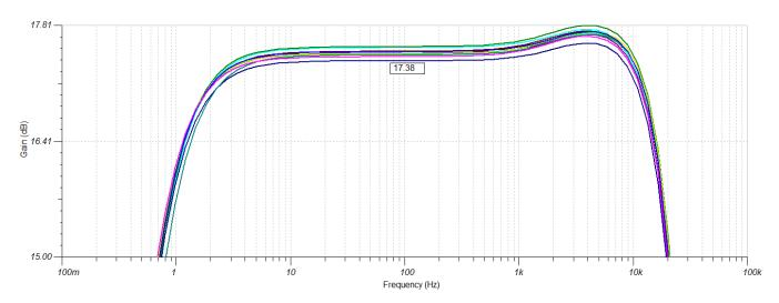
图 15. Signal Chain Passband at +12-dB Gain Setting
