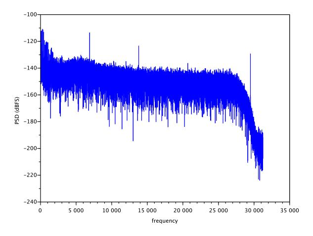
图 25. Noise in Presence of Image Frequency at 8.01 MHz
