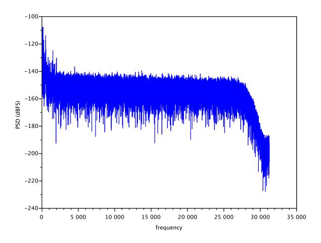
图 26. Noise Floor With External Sensor Simulator Connected
