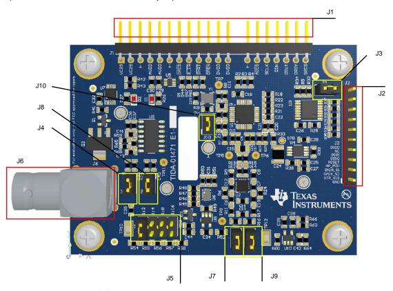
图 19. TIDA-01471 PCB Hardware—Top View
