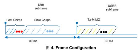
注: The design uses a fixed profile and changing the parameters requires the user to update the code. The main configuration header is /common/srr\_config\_consts.h. Find the SRR configuration in /common/srr\_config\_chirp\_design\_SRR80.h and the USRR configuration is available in /common/ srr\_config\_chirp\_design\_USRR20.h. The design (and intent) of the two subframes are provided as follows.
