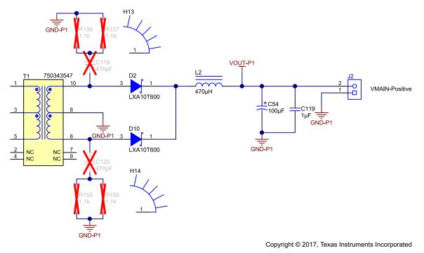
图 12. Output Rectifier and Filtering for Positive Output
