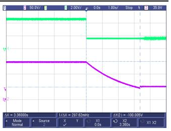
图 73. +HV-Out (Turnoff) From 150 to 50 V at Full Load
