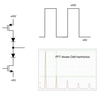
图 4. Pulser—Output Waveform and FFT of Output
