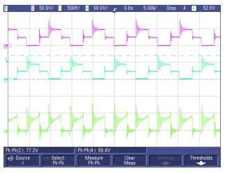
图 60. MOSFET Stress VDS for -HV Output
