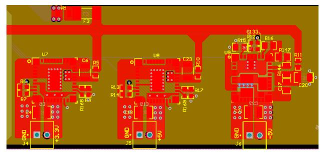
图 103. Layout for LMZ Modules
