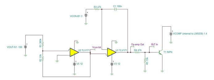
图 18. TINA Simulation for Feedback Circuit for Negative Rail for HV Section
