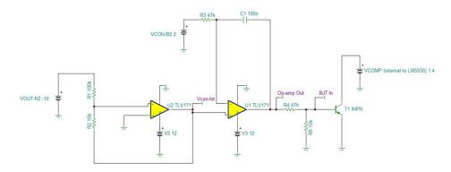
图 24. TINA Simulation for Feedback Circuit for Negative Rail for LV or MID Section
