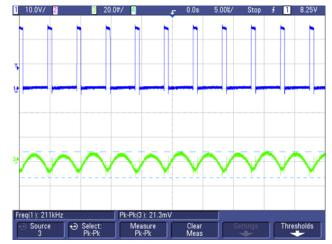
图 89. SW Node Waveform and Output Ripple for Vout = 3.3 V, Iout = 1 A
