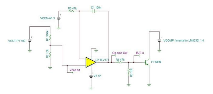
图 15. TINA Simulation for Feedback Circuit for Positive Rail for HV Section
