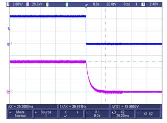
图 77. +LV/Mid-Out (Turnoff) From 50 to 0 V at Full Load
