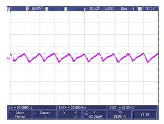
图 64. Output Voltage Ripple for +LV or MID Output at Full load
