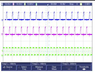
图 97. External SYNC Clock = 300 kHz (Channel 3 in Green)
