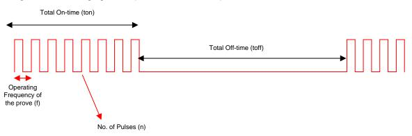
图 43. Load Profile for Testing TIDA-01352 in Different Imaging Modes
