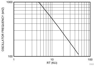
图 9. LM5030 Oscillator Frequency versus RT
