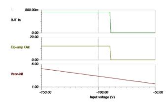
图 19. Simulation Waveform Showing Linearity (-HV Output)
