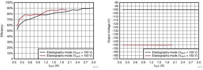
图 55. Elastography Mode Efficiency (-HV Output)
