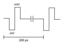
图 6. Three-Level Pulser Output Waveform
