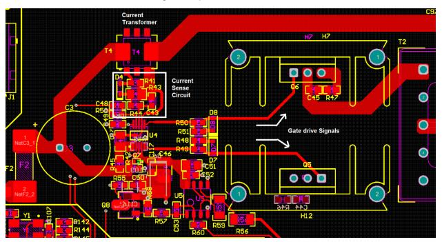
图 102. Routing for CS Pin for LM5030
