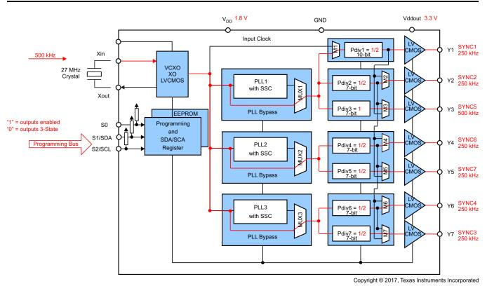
图 42. Clock Programming for Synchronization of All Devices to  $f_{IN}$  = 500 kHz
