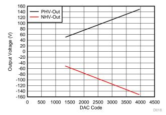
图 68. Output Voltage Linearity for U11 With Respect to Digital Input Code
