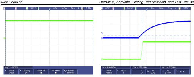
图 82. V<sub>out</sub> = 5 V at V<sub>IN</sub> = 24 V
