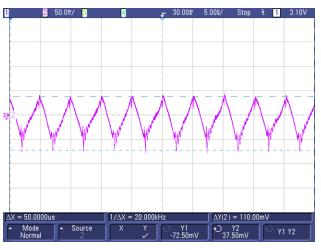
图 52. Output Voltage Ripple for +HV Output
