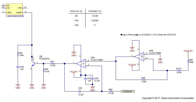
图 17. Feedback Circuit for Negative Rail for HV Section
