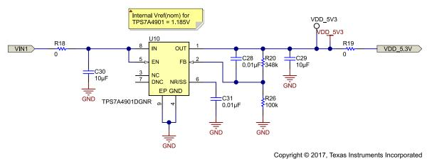
图 27. Power Supply for DAC60004
