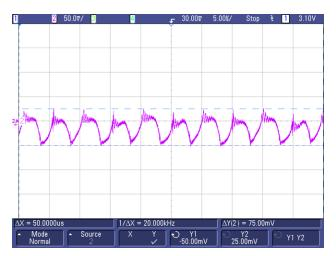
图 61. Output Voltage Ripple for –HV Output
