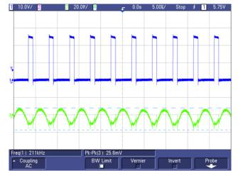
图 84. SW Node Waveform and Output Ripple for  $V_{\text{out}}$  = 5 V,  $I_{\text{out}}$  = 1 A
