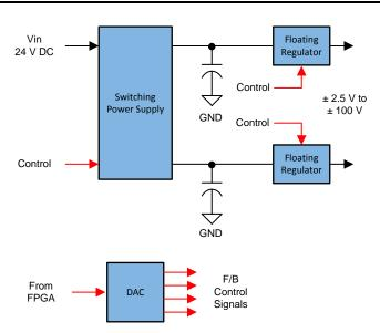
图 3. Typical Power Supply Scheme in Medical Ultrasound Application
