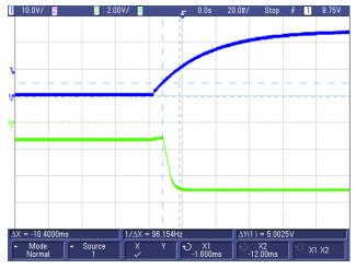
图 93. Start-up Waveform (for  $V_{out} = -5$  V) Showing Soft-Start Time = 10.4 ms
