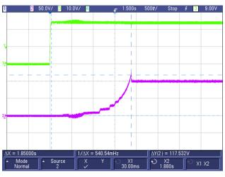
图 50. Start-up Waveform for +HV Output
