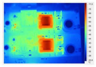
图 70. Thermal Image for ±HV Sections
