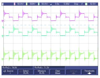
图 51. MOSFET Stress VDS for +HV Output
