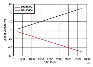
图 69. Output Voltage Linearity for U12 With Respect to Digital Input Code
