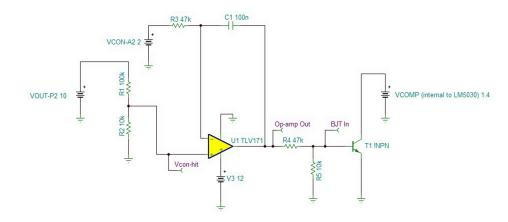
图 21. TINA Simulation for Feedback Circuit for Positive Rail for LV or MID Section
