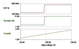
图 16. Simulation Waveform Showing Linearity (+HV Output)
