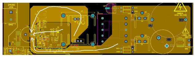
图 101. Star Ground Topology for Power Supply
