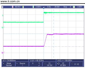
图 72. +HV-Out (Turnon) From 50 to 150 V at Full Load
