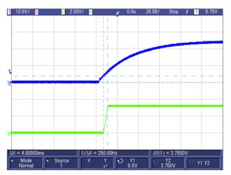
1 88. Start-up Waveform (for V\_{out} = 3.3 V) Showing Soft-Start Time = 4 ms
