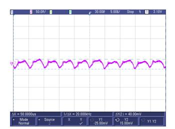
图 67. Output Voltage Ripple for –LV or MID Output at Full load
