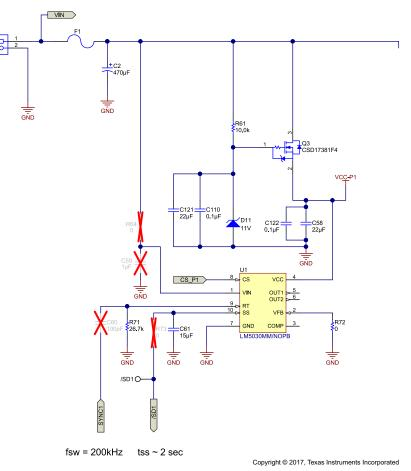
图 8. Input Section and Turnon Mechanism for LM5030
