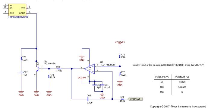
图 14. Feedback Circuit for Positive Rail for HV Section
