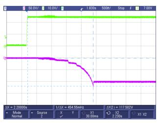
图 59. Start-up Waveform for –HV Output
