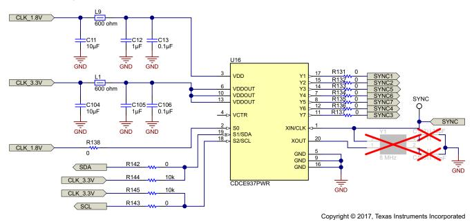
图 34. Schematic Capture for CDCE937—Clock SYNC Buffer
