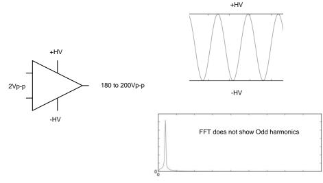
图 5. Linear Amplifier—Output Waveform and FFT of Output
