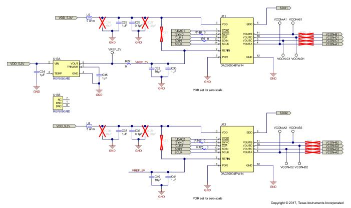
图 26. DAC60004 to set up Outputs for Power Supplies
