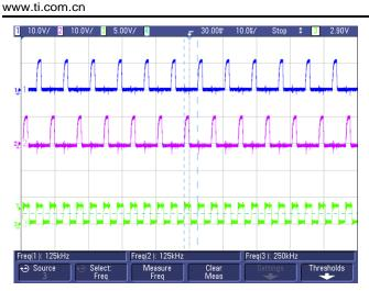
图 96. External SYNC Clock = 250 kHz (Channel 3 in Green)
