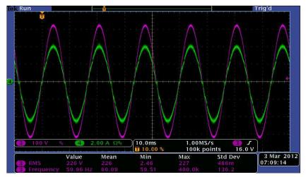
(1) Ch3 -Vin, Ch4-lin, Vrms=230V, Vbus=390V, Pout=700W
