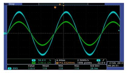
图 14. IL PFC Input Voltage and Current at 550W Load and 110Vrms Input
