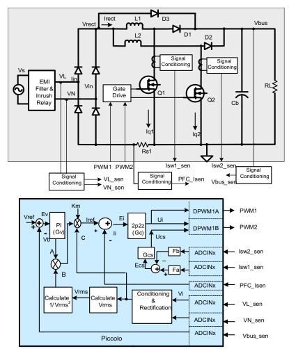
图 3. Interleaved PFC Converter Control Using the C2000 Microcontroller
