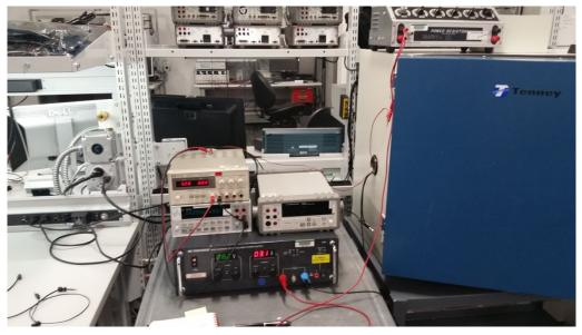
图 16. Primary Side Functional Test Setup
