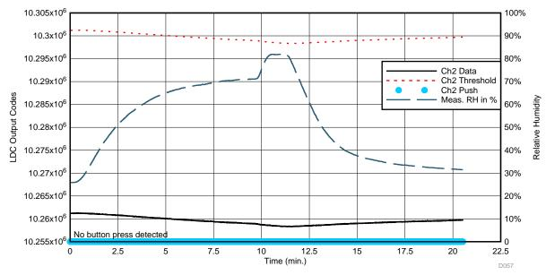
图 52. LDC Ch2 Data During Relative Humidity "Shock" Test—Big Button Channel
