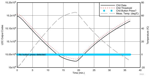
图 45. LDC Ch0 Data During Thermal "Shock" Test—Down Button Channel
