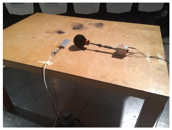
图 56. IEC 61000-4-3 Radiated Immunity Test Setup
