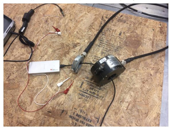
图 83. IEC 61000-4-6 Conducted Immunity Test Setup
