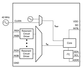
图 5. LDC1614 Functional Block Diagram
