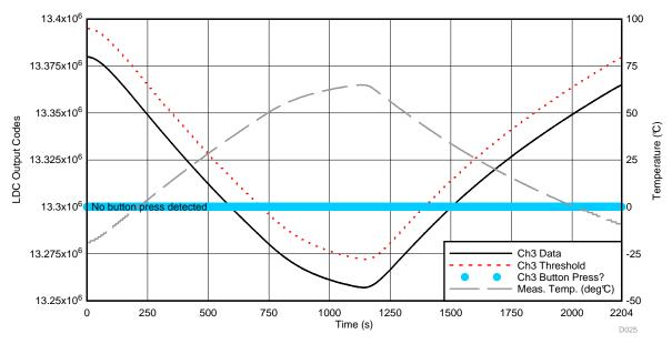
图 48. LDC Ch3 Data During Thermal "Shock" Test—Little Button Channel
