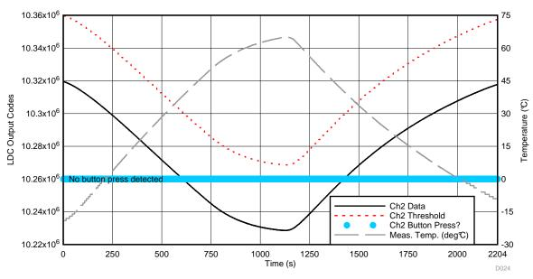
图 47. LDC Ch2 Data During Thermal "Shock" Test—Big Button Channel
