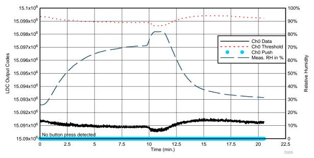
图 50. LDC Ch0 Data During Relative Humidity "Shock" Test—Down Button Channel
