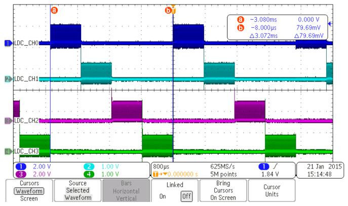
图 22. LDC1614 Measurement Sequence
