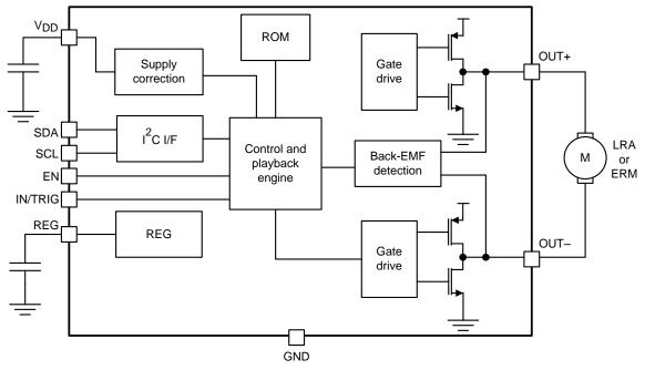
图 6. DRV2605L Functional Block Diagram
