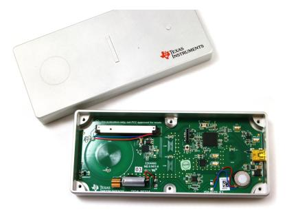
图 2. Touch on Metal Buttons With Integrated Haptic Feedback Mechanical Enclosure Detail
