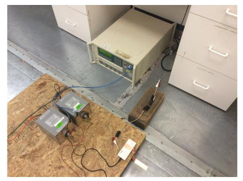
图 74. IEC 61000-4-5 Surge Test Setup
