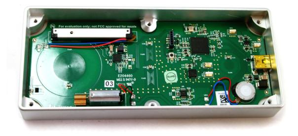
图 14. Touch on Metal Buttons With Integrated Haptic Feedback Reference Design Hardware
