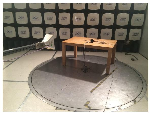
图 55. IEC 61000-4-3 Radiated Immunity Test Setup
