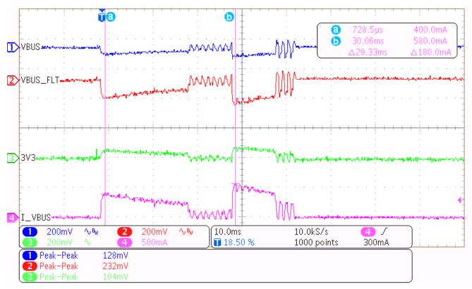
图 41. Power Data During ERM Actuator Operation
