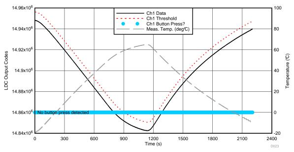
图 46. LDC Ch1 Data During Thermal "Shock" Test—Up Button Channel
