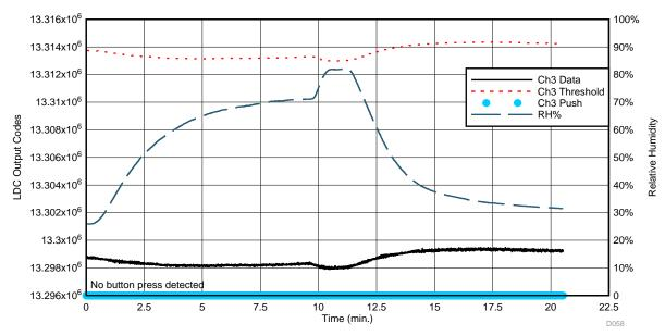
图 53. LDC Ch3 Data During Relative Humidity "Shock" Test—Little Button Channel
