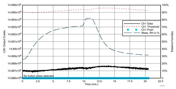
图 51. LDC Ch1 Data During Relative Humidity "Shock" Test—Up Button Channel
