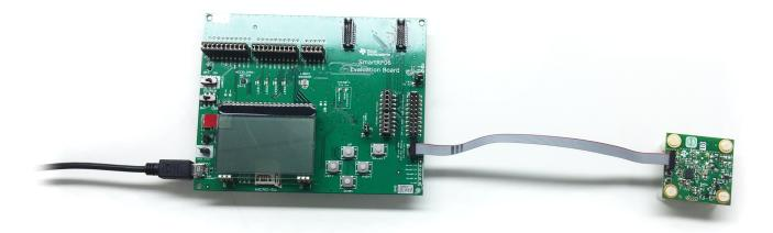
图 10. Connection of SmartRF06 Evaluation Board and TI Designs Hardware for Programming/Debugging
