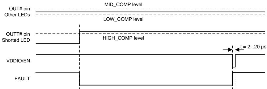
Figure 17. LED Short Fault
