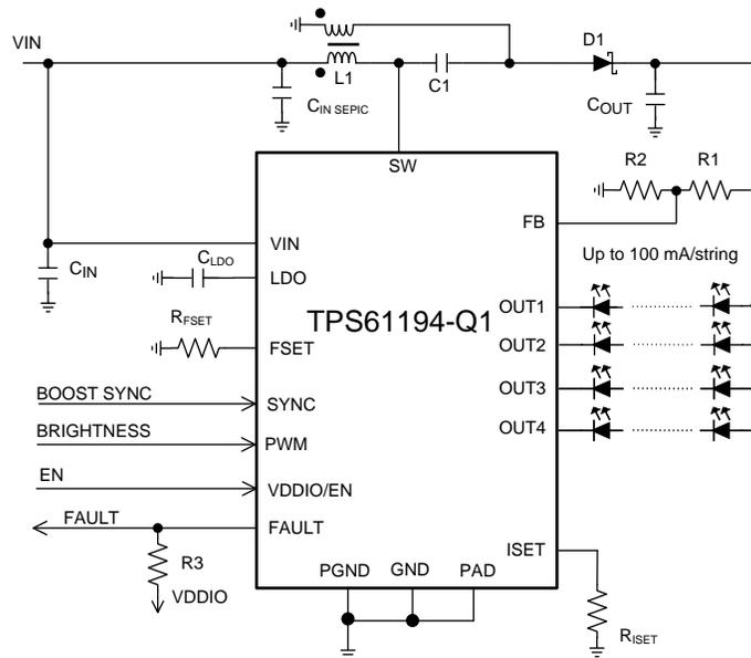
Figure 25. SEPIC Mode, 4 Strings, 100 mA per String Configuration
