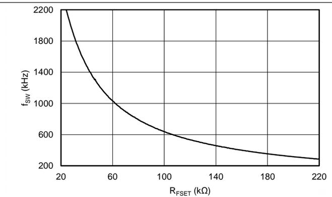
Figure 6. Boost Switching Frequency  $f_{SW}$  vs  $R_{ISET}$
