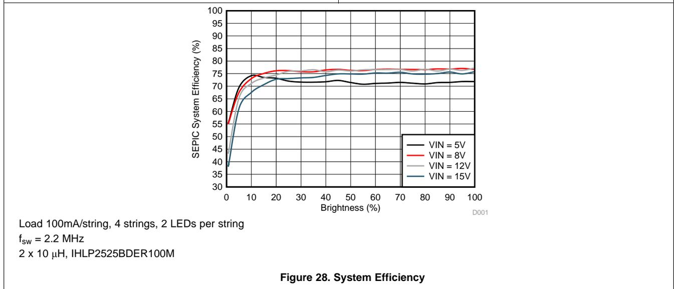
Figure 28. System Efficiency
