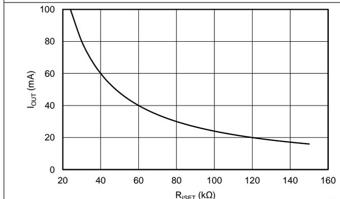
Figure 5. LED Current vs  $R_{ISET}$
