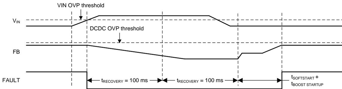
Figure 14.  $V_{IN}$  Overvoltage Protection ( $V_{IN}$  OVP)
