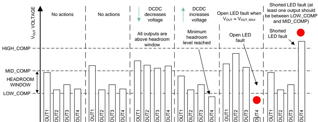
Figure 12. Protection and DC-DC Voltage Adaptation Algorithms
