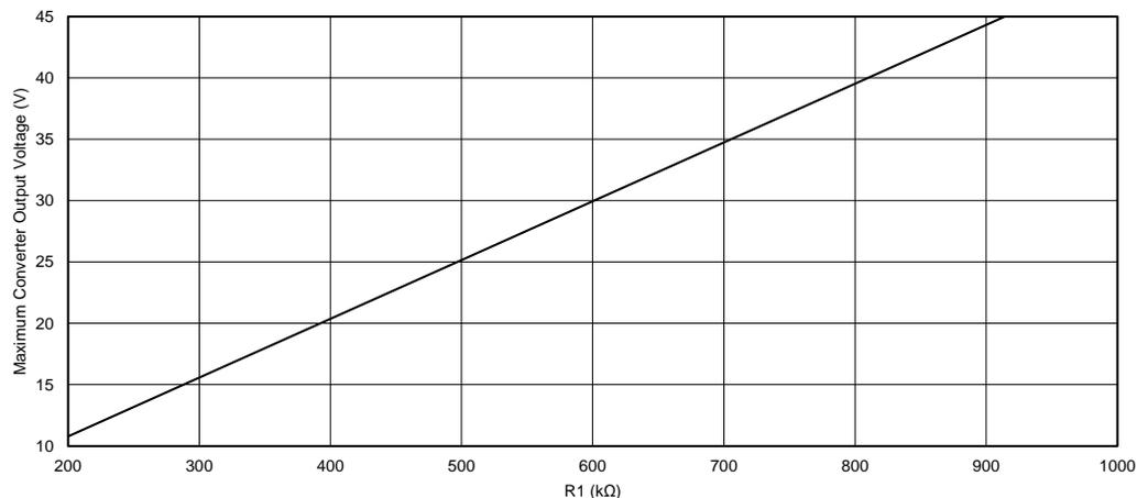
Figure 9. Maximum Converter Output Voltage vs R1 Resistance
