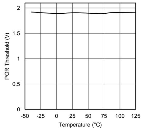
Figure 5. POR Threshold vs Temperature
