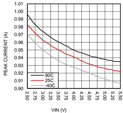
Figure 51. Open Loop Current Limit vs.  $V_{IN}$
