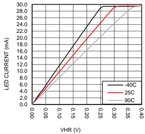
Figure 49.  $H_{VLED}$  Current vs. Current Sink Headroom Voltage
