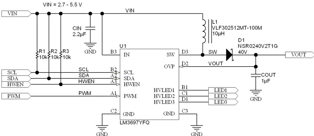
Figure 13. LM3697 Schematic
