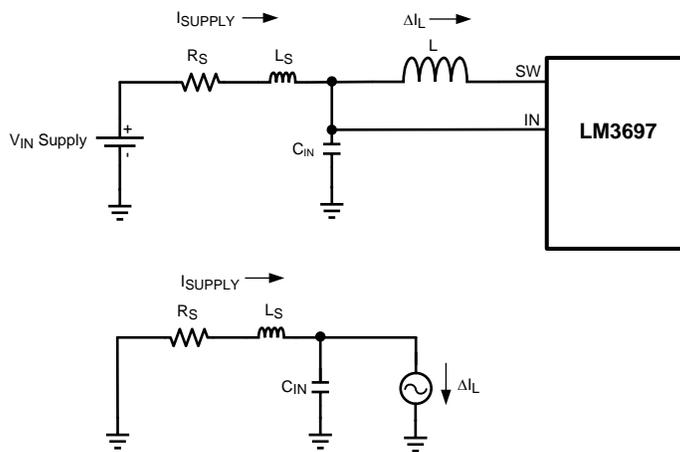
$$1. \frac{1}{L_S \times C_{IN}} > \frac{R_S^2}{4 \times L_S^2}$$
