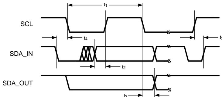
Figure 1. I<sup>2</sup>C-Compatible Interface Timing
