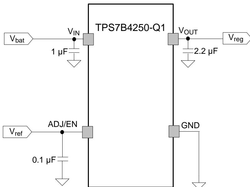
**Figure 16. Typical Application Schematic**
