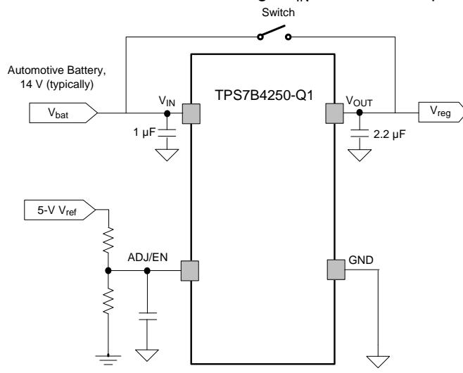
**Figure 13. Output-Voltage Short to Battery**
