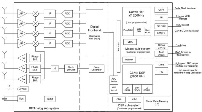
Figure 2. IWR6843 mmWave Sensor Functional Block
