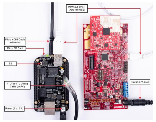
Figure 10. TIDEP01013 Gesture HMI Hardware Setup
