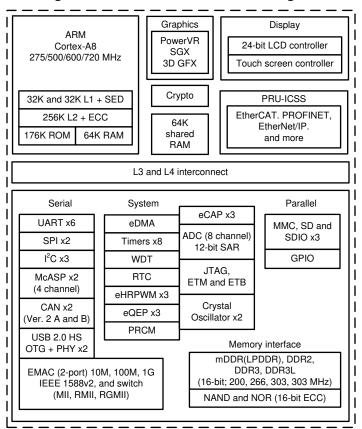
Figure 1. AM335x Processor Block Diagram
